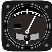
Right turn no slip/skid
