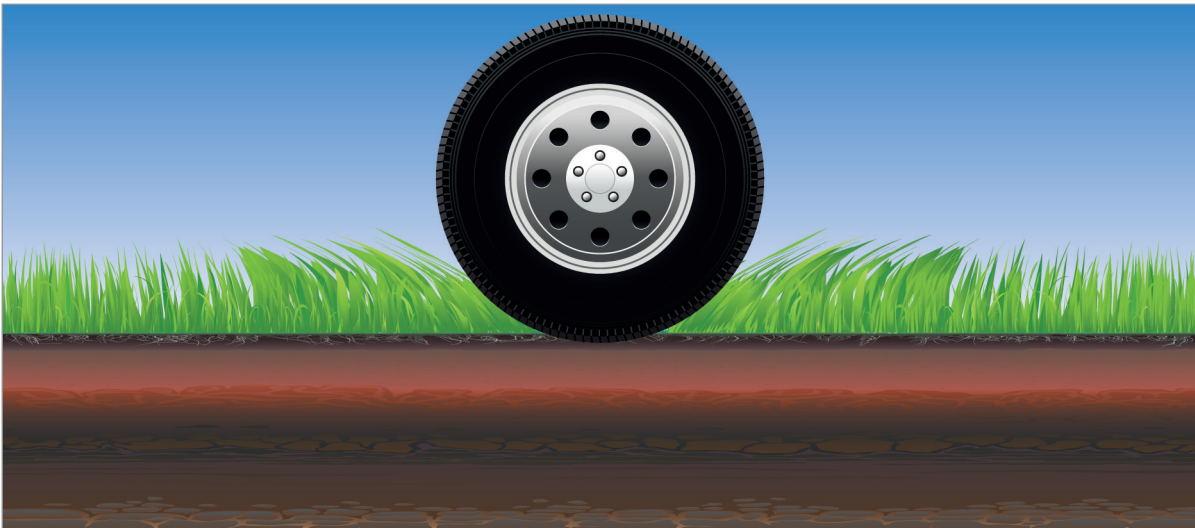
Figure 6.6 An illustration showing that for the wheel to advance grass must be pushed out of the way
