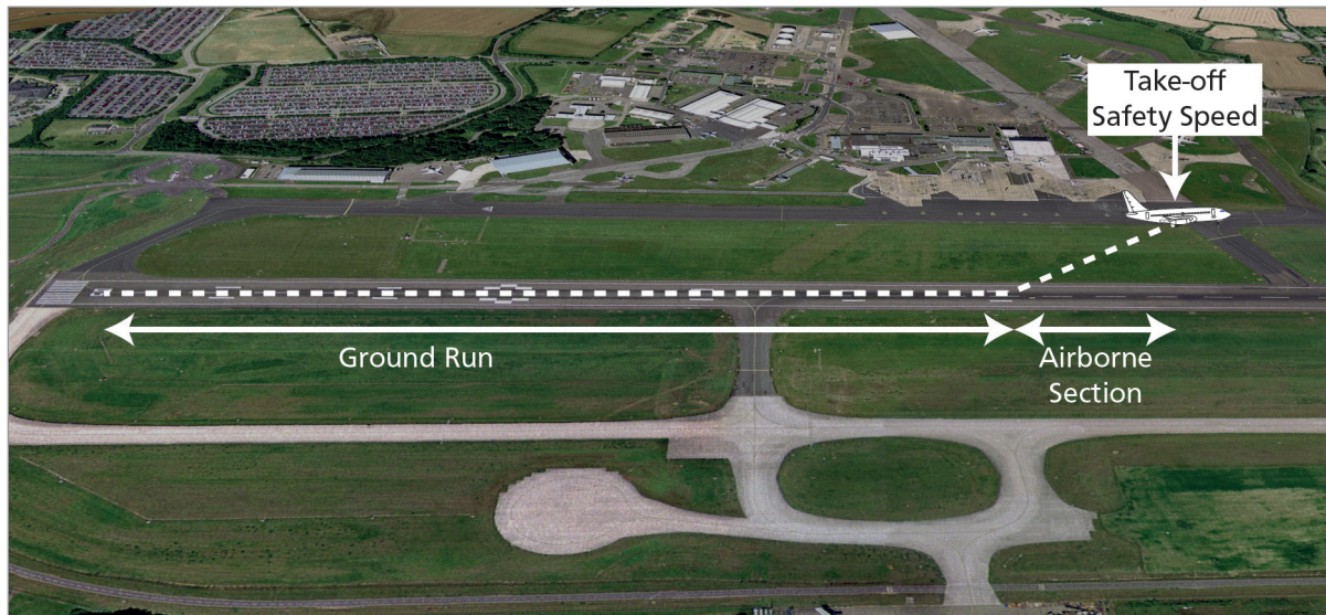
Figure 2.5 The take-off distance (TOD) is the total distance from brake release until the screen height
