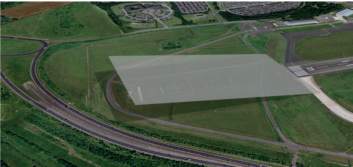
Figure 2.1 Clearways extend from the end of the runway with an upward slope not exceeding 1.25%, above which no object or terrain protrudes
