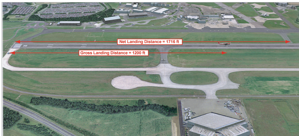
Figure 10.2 To obtain the minimum length of runway required, multiply the gross landing distance by 1.43.
