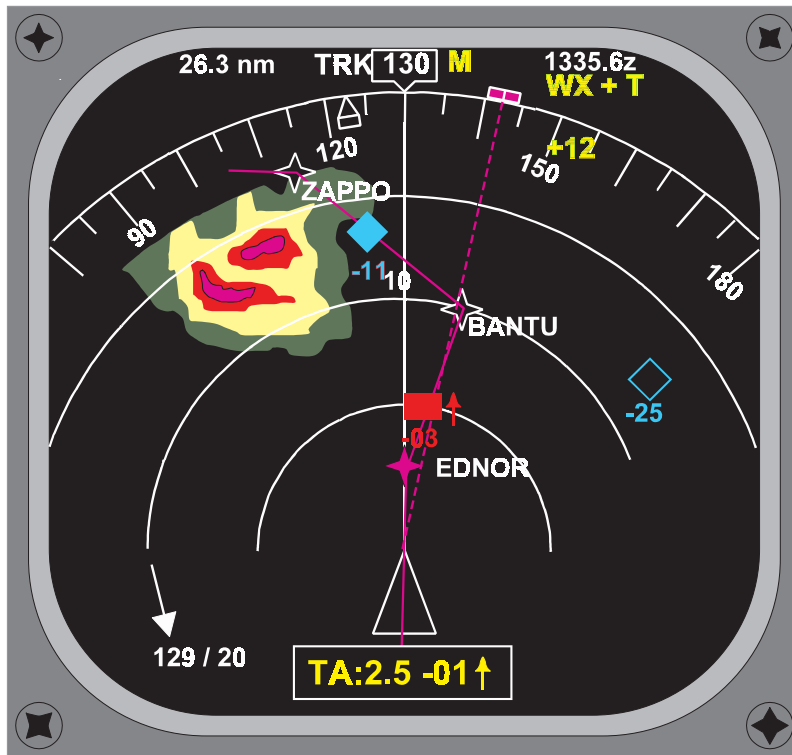
Figure 35.8 Navigation display in MAP mode showing TCAS
