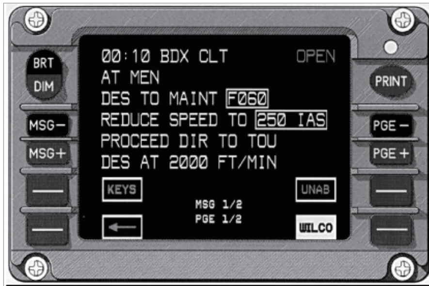
Figure 24.5 The diagram shows a typical DCDU message display
