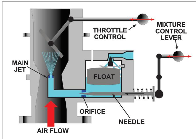
Figure 8.7 A needle type mixture control.
