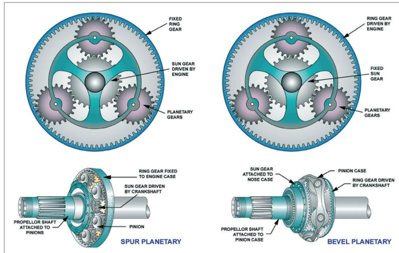
Figure 12.23 Spur & bevel planetary gears
