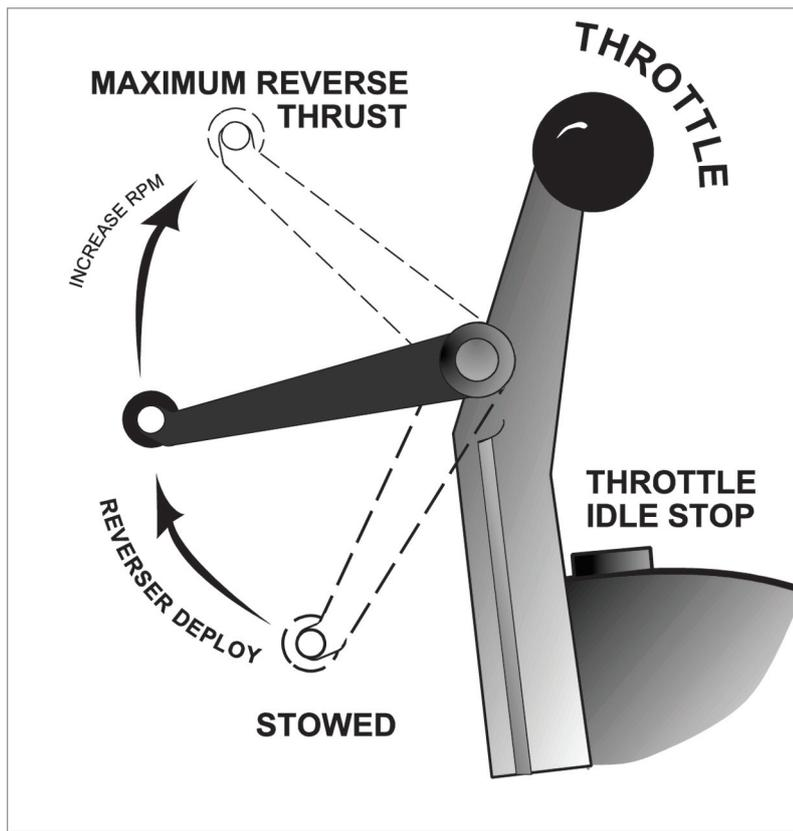
Figure 21.2 Throttle & reverse thrust lever.
