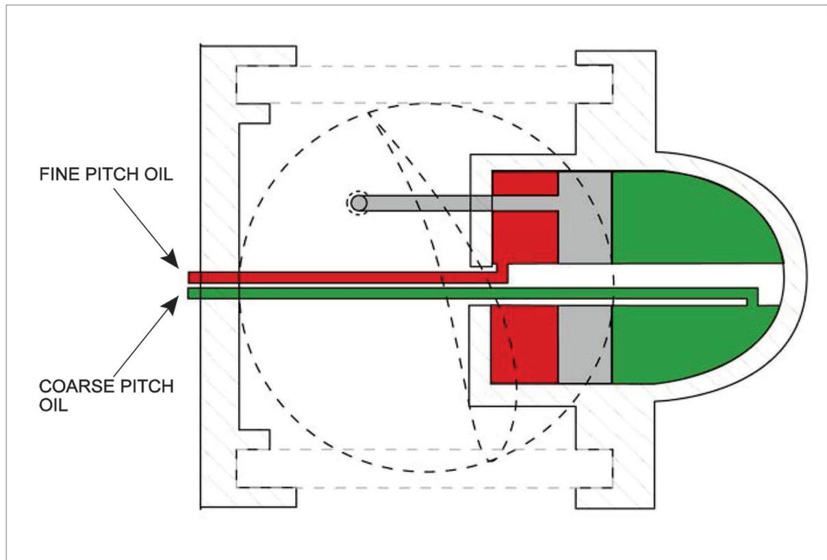
Figure 12.10 The double acting propeller.
