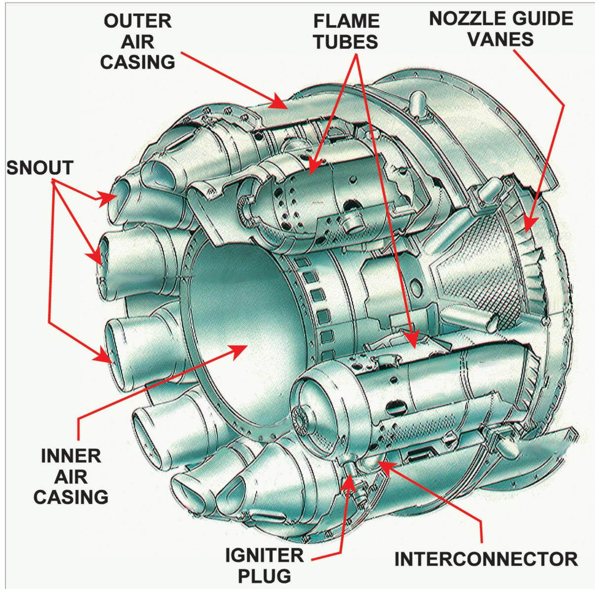
*Figure 16.4* A turbo-annular combustion chamber system.
