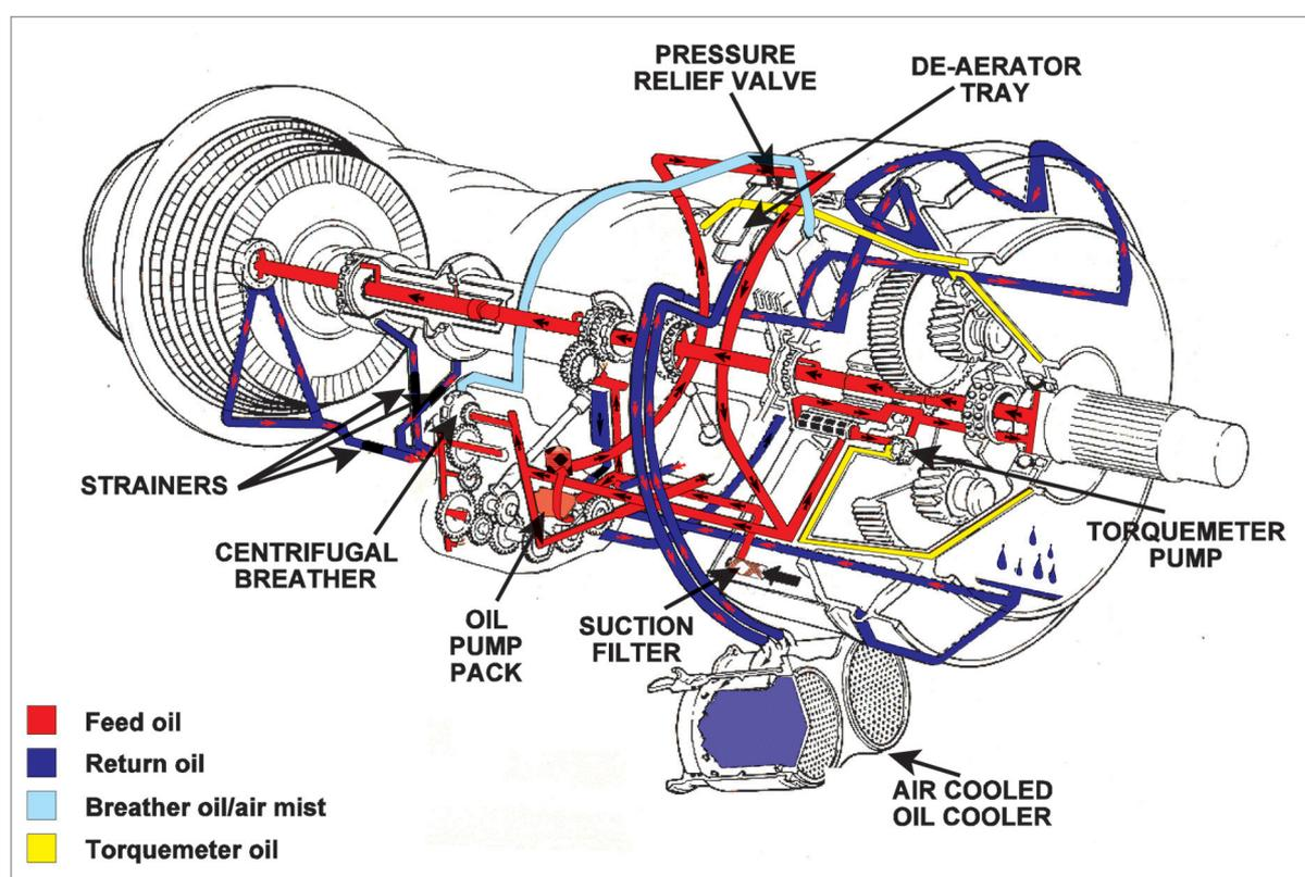
Figure 19.2 A pressure relief valve type oil system.
