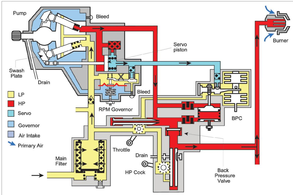
Figure 26.3 Hydro-mechanical fuel control
