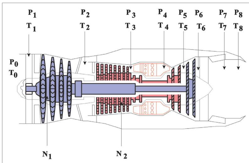
*Figure 13.10 A twin spool low ratio bypass turbojet*
