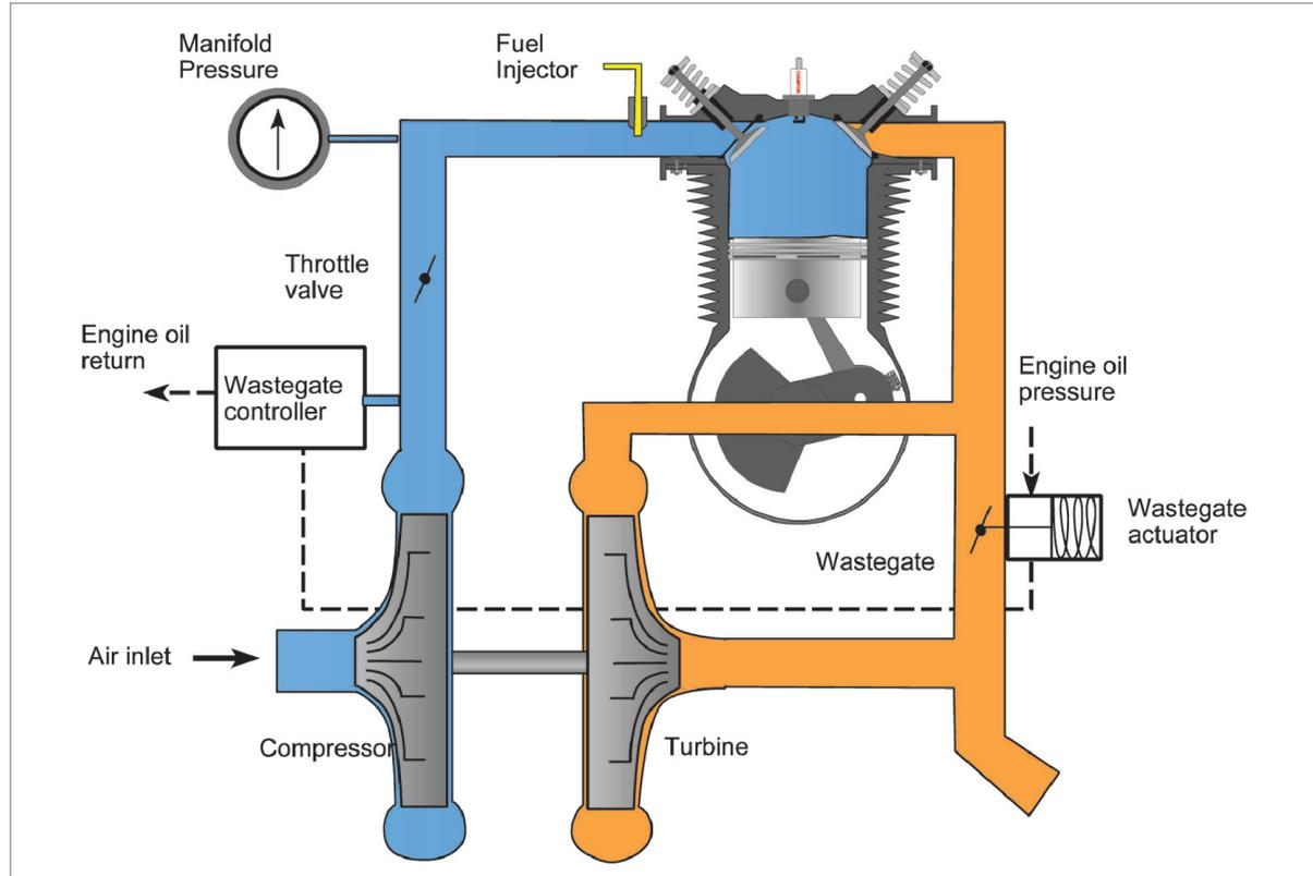
Figure 11.3 Turbocharger - general arrangement.
