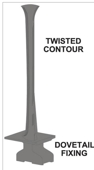
*Figure 15.7 A typical compressor rotor blade.*
