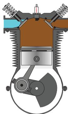
**4. The exhaust valve is now open to atmosphere. The piston moving up forces the exhaust gas past it to the atmosphere. The atmosphere provides a resistance to the flow of exhaust gas which is termed 'EXHAUST BACK PRESSURE'. Because of this the pressure in the cylinder increases slightly which causes the temperature to rise also.**
