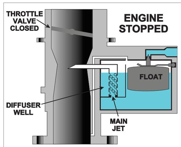
Figure 8.4 A diffuser well fitted in a carburetor float chamber.
