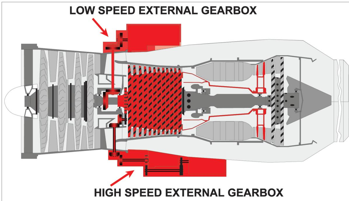
Figure 22.3 Spreading the load of accessories between two gearboxes.
