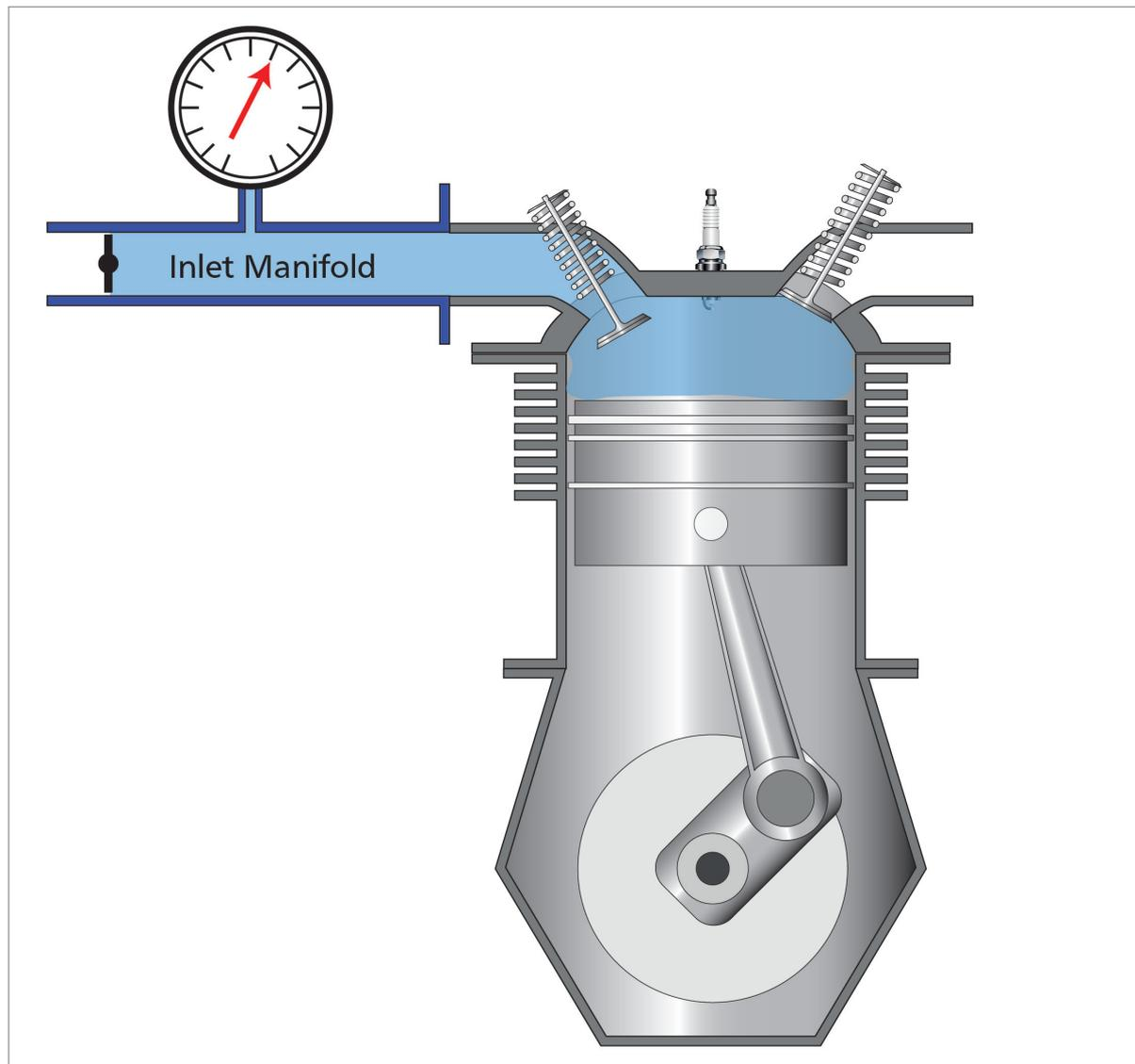
*Figure 2.8* Manifold absolute pressure gauge
