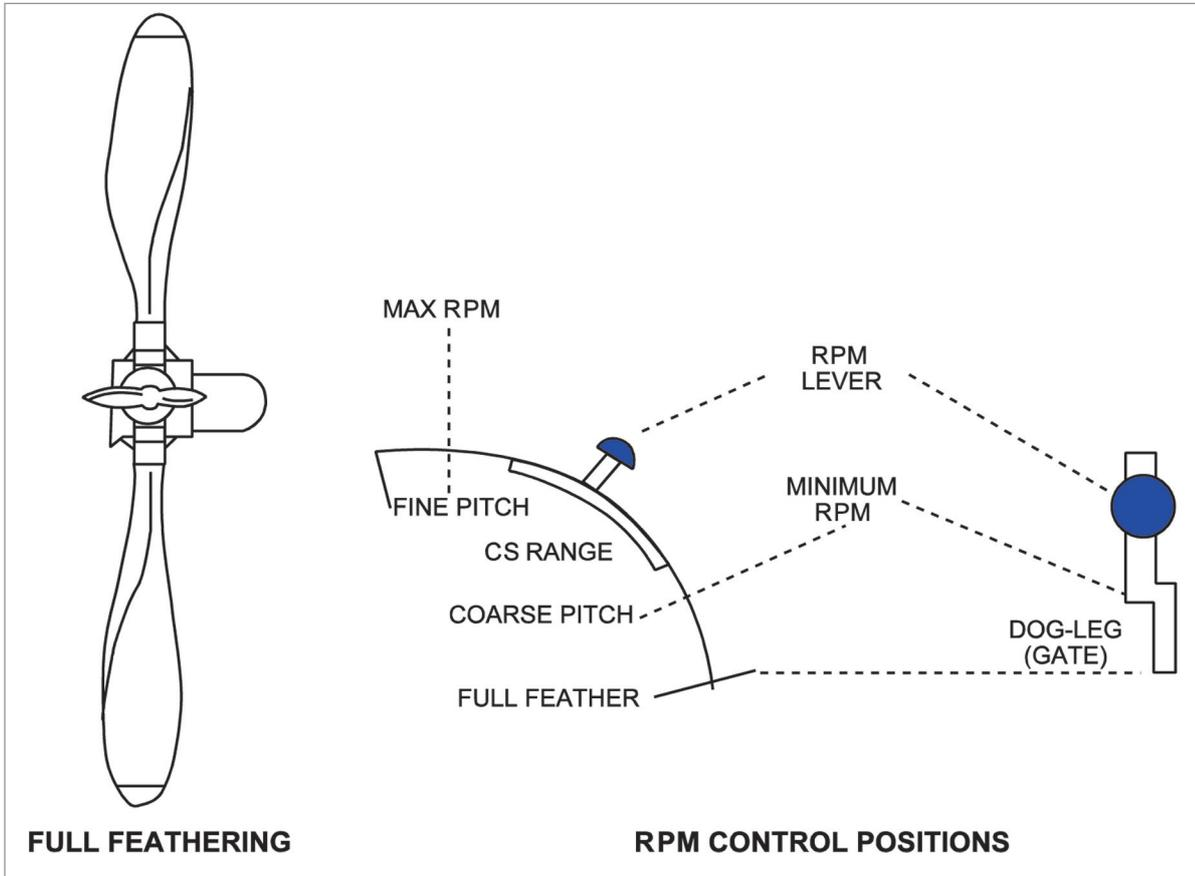
Figure 12.16 Feathered propeller & prop control gate showing feather.
