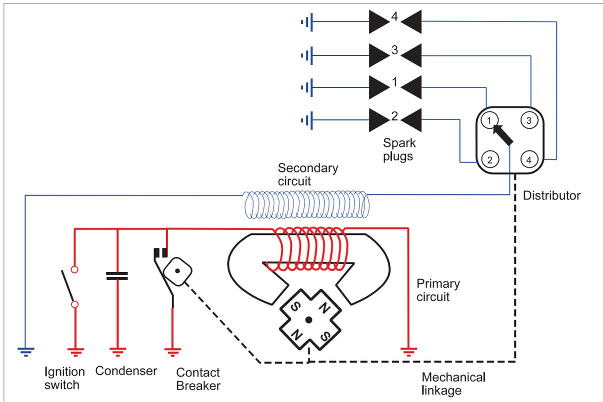
Figure 5.1 Magneto Circuit
