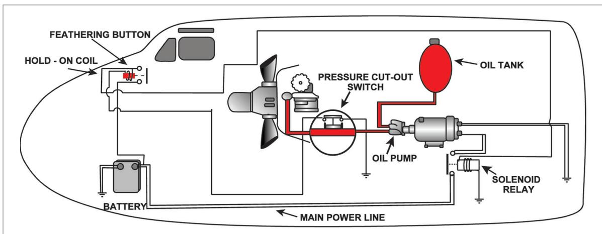
Figure 12.18 Typical feathering installation.
