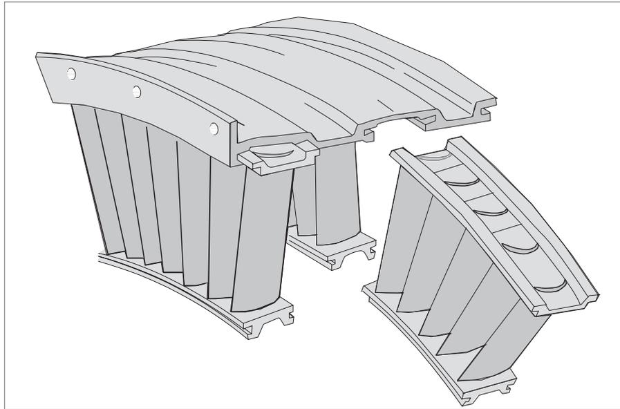
Figure 15.8 Segments of shrouded stator vanes.
