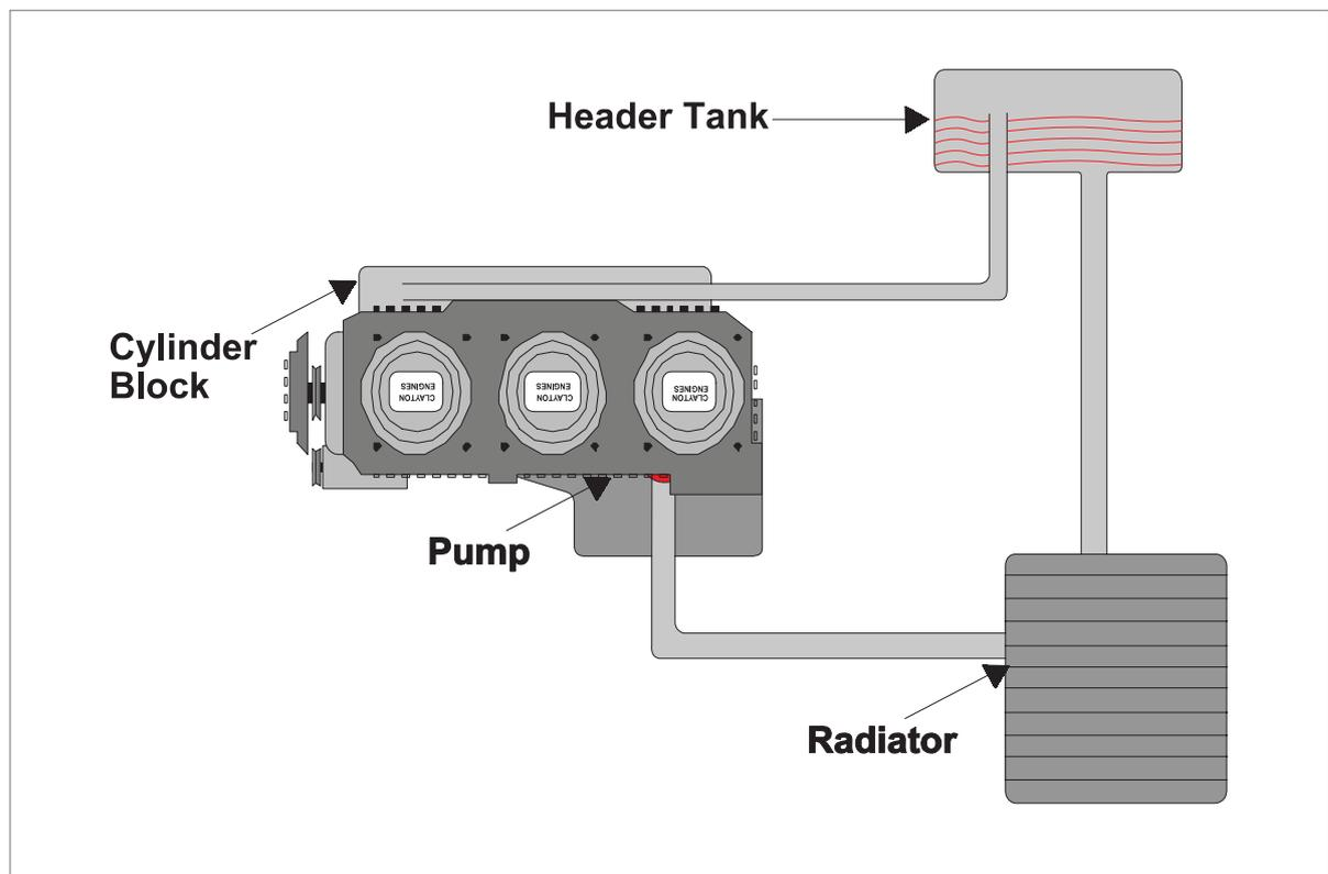
*Figure 4.1 Liquid cooling system.*
