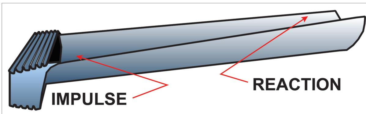
Figure 17.4 The combination impulse-reaction blade.
