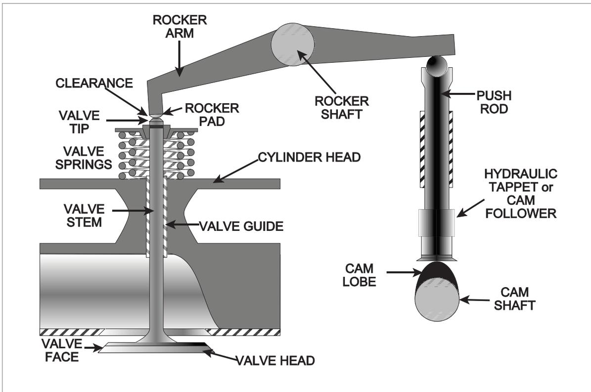
Figure 2.15 Valve clearance
