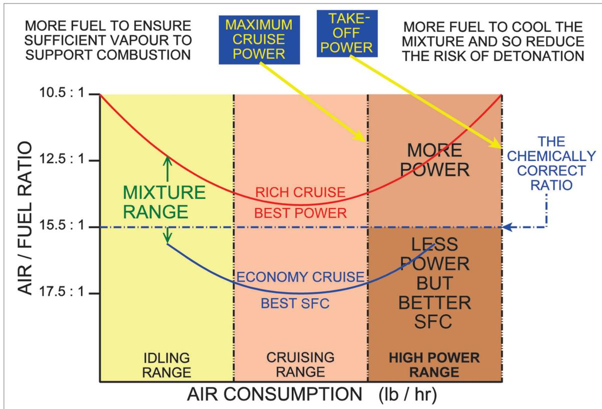
Figure 7.1 A typical air/fuel mixture curve.
