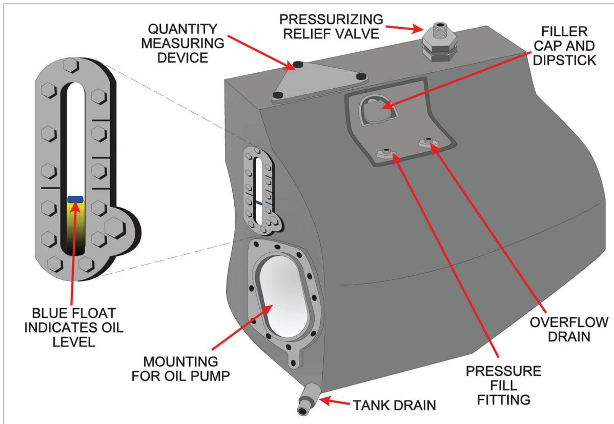
Figure 19.4 A typical oil tank.
