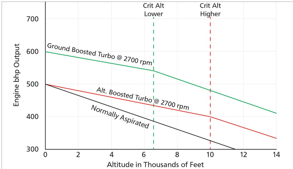
Figure 11.6 A comparison of the power curves of a normally aspirated engine & a turbocharged engine.
