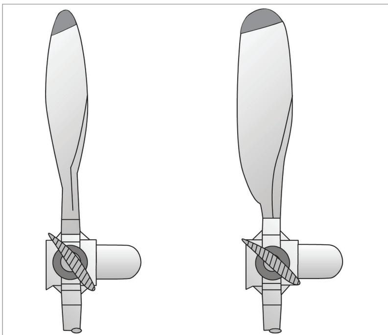
Figure 12.11 Propeller with various pitch angles.
