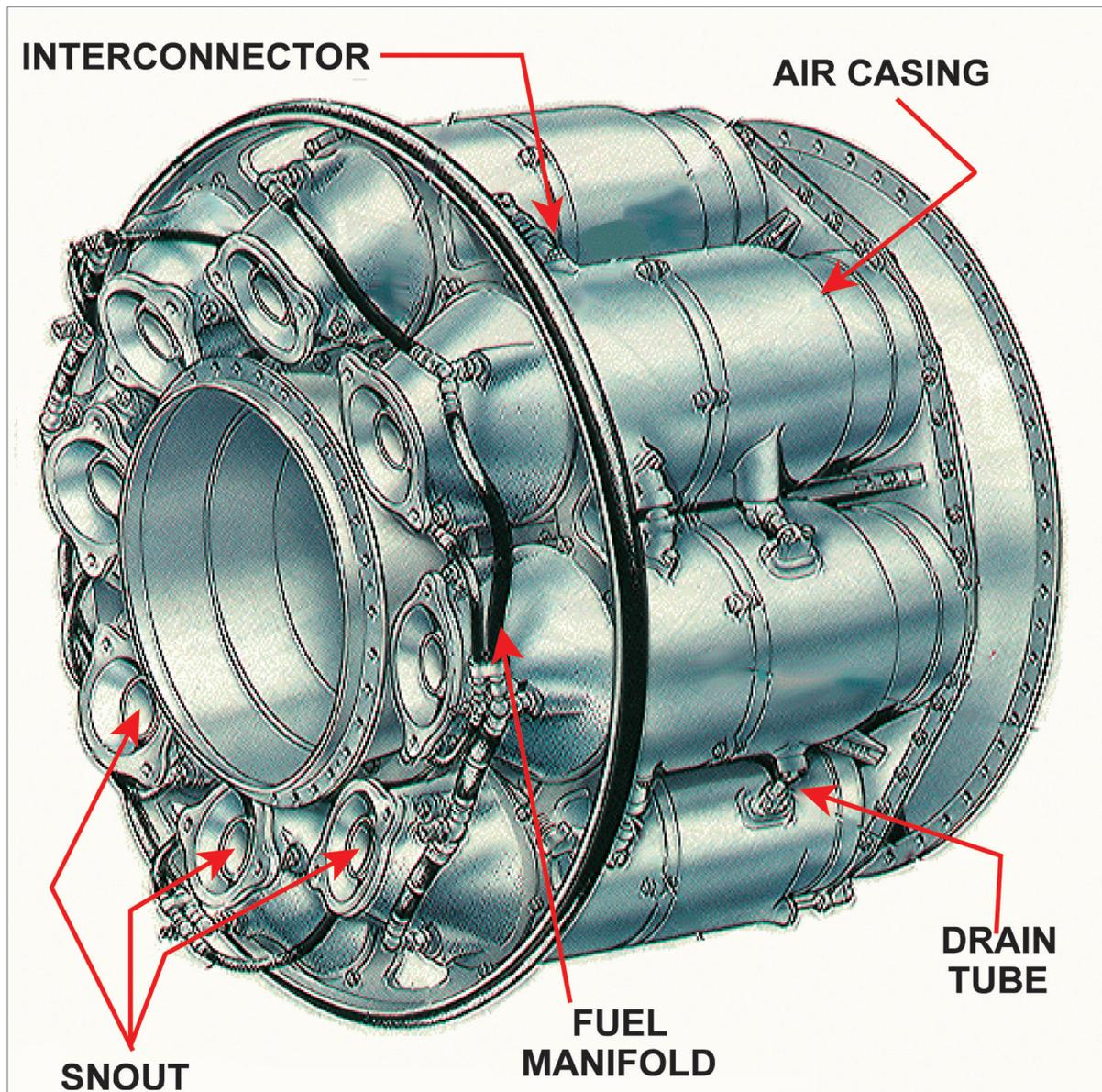
*Figure 16.3 A multiple combustion chamber system.*
