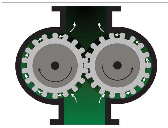
Figure 19.5 A gear type oil pump.
