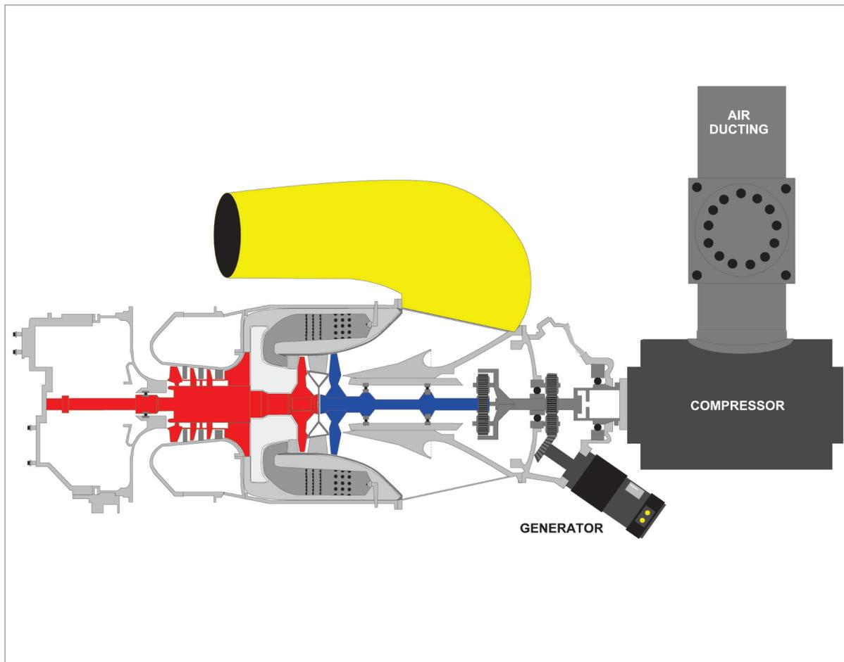
Figure 24.1 Free turbine turboshaft APU
