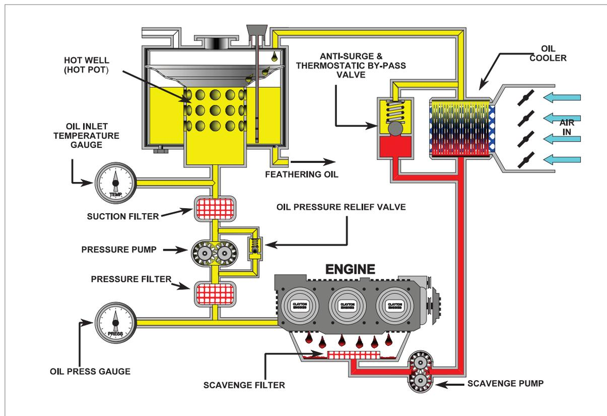
Figure 3.1 Dry sump lubrication
