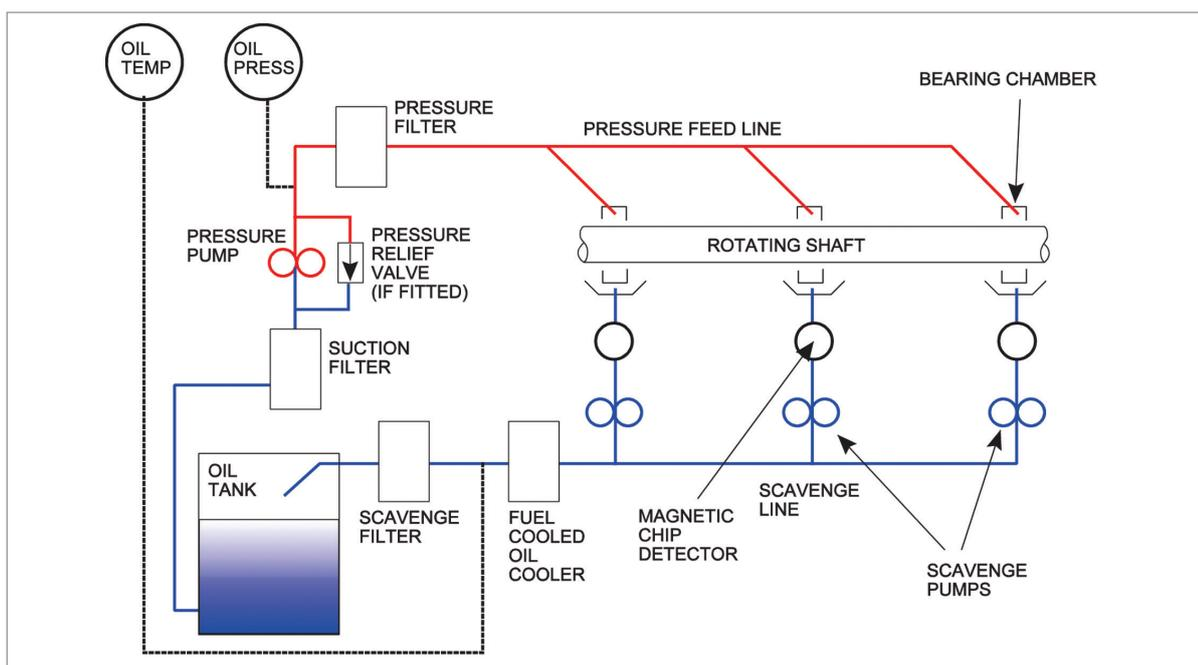
Figure 19.1 Schematic gas turbine oil system.
