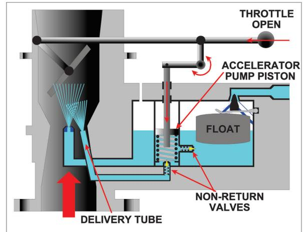
*Figure 8.11 An accelerator pump.*
