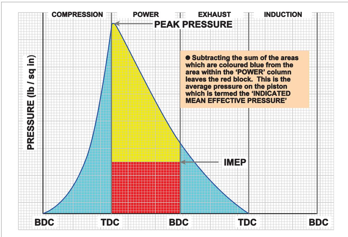
Figure 2.9 An indicator diagram plotted against stroke for simpler calculation of pressure areas
