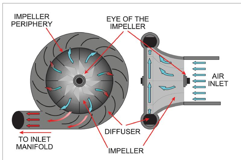
*Figure 11.1 A centrifugal compressor.*
