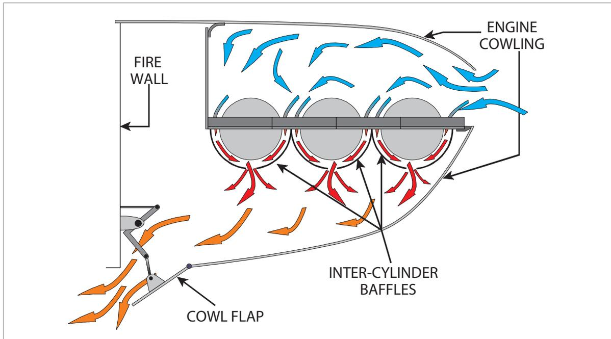
Figure 4.2 Cooling airflow in a six cylinder horizontally opposed engine.
