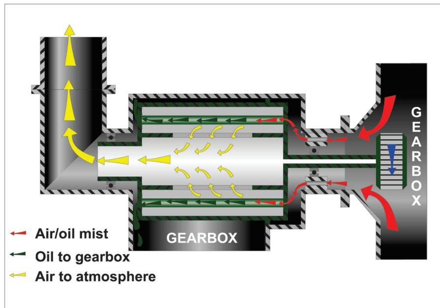
*Figure 19.8 The centrifugal breather & vent.*
