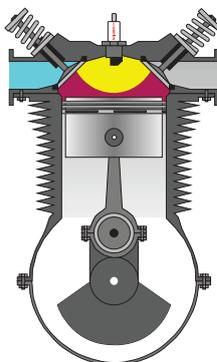
**3. Both valves are still closed. The piston is stationary at the top of the stroke (TDC) The temperature of the charge is increasing rapidly during combustion. The VOLUME IS UNCHANGED due to the stationary piston, hence the internal combustion engine is known as a 'CONSTANT VOLUME ENGINE'.**
