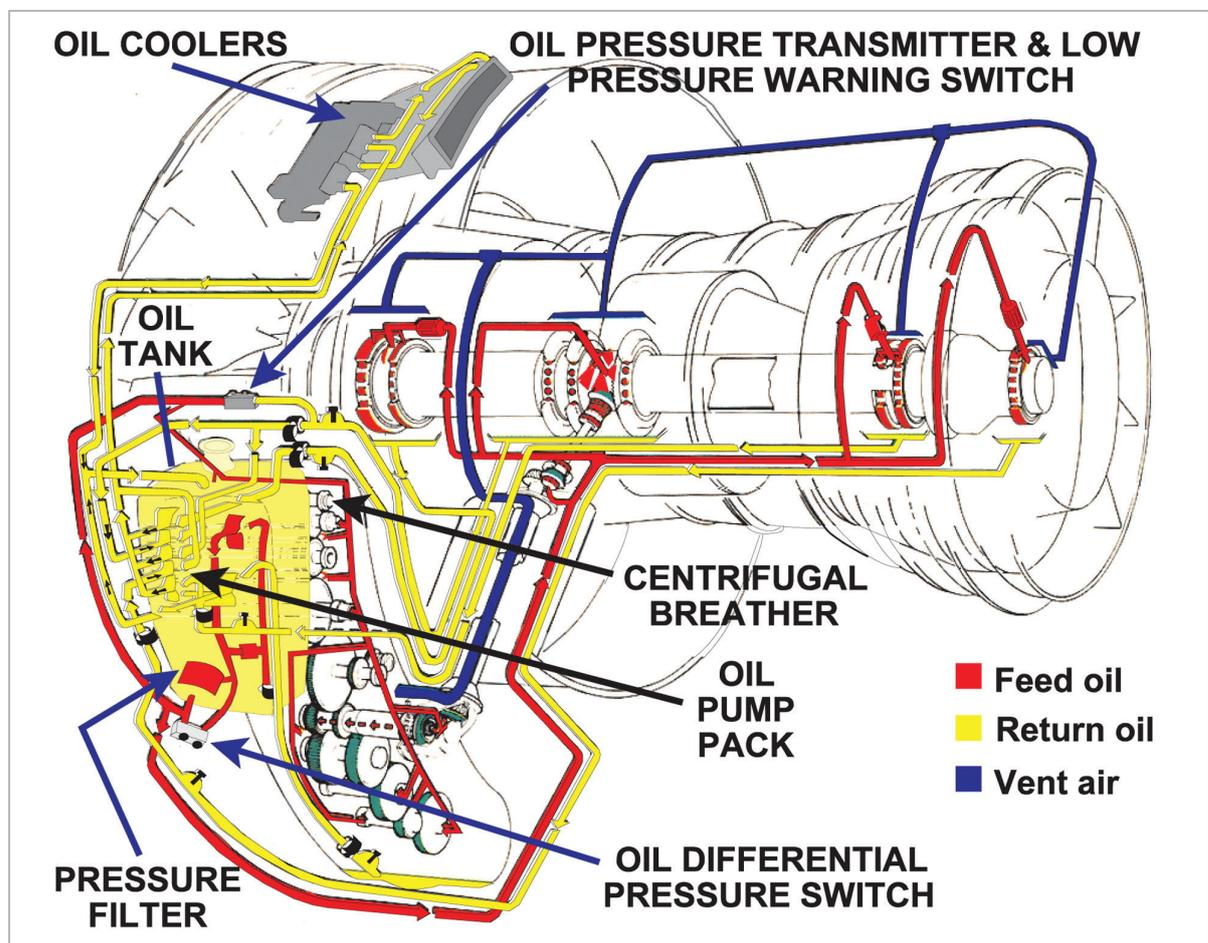
Figure 19.3 A full flow type lubricating system.
