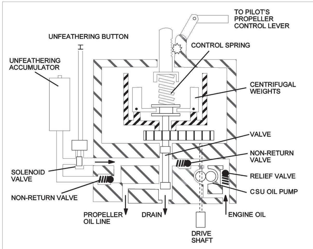
Figure 12.17 CSU with unfeathering accumulator
