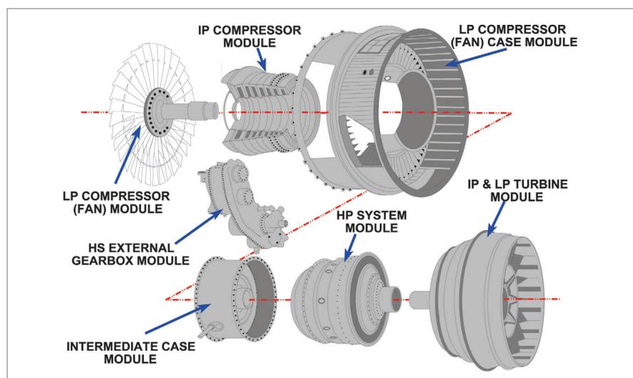
*Figure 13.13 Modular construction units.*
