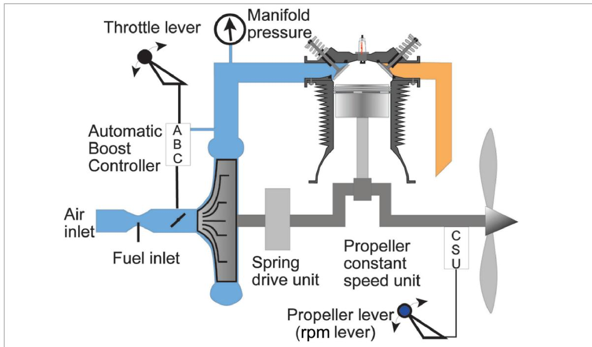
Figure 11.9 Internally driven supercharger - general arrangement.
