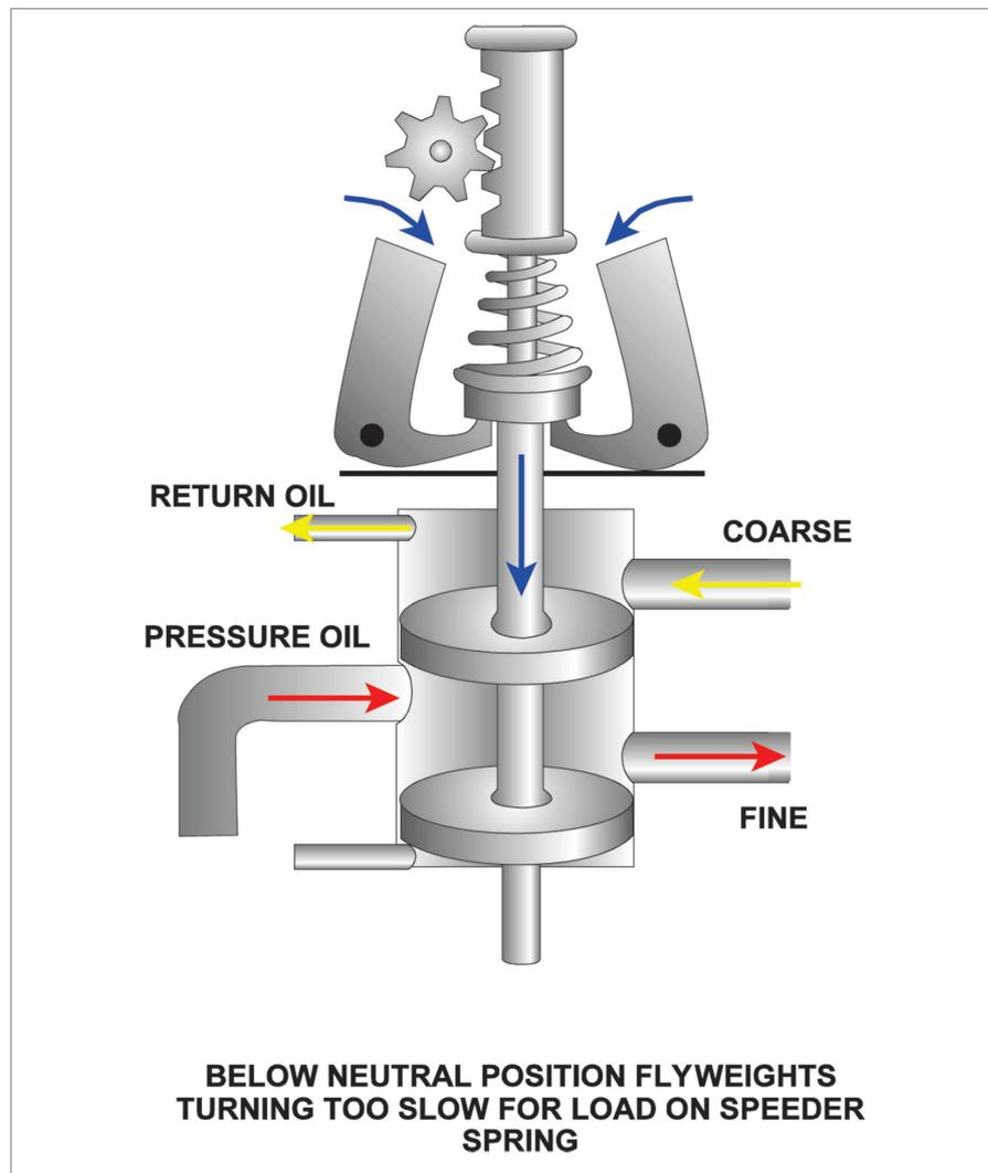
Figure 12.14 Underspeed condition.
