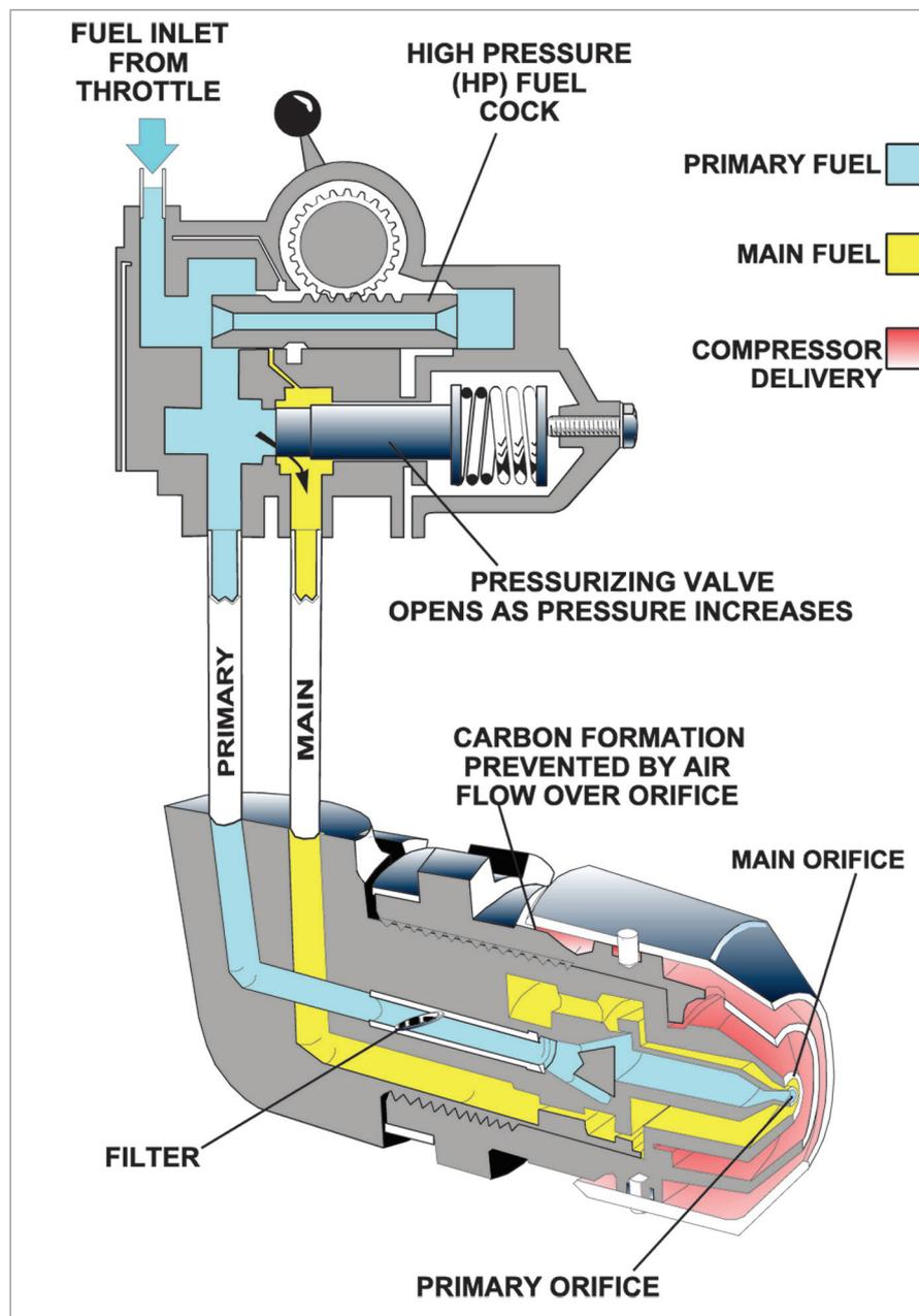
Figure 16.12 The duplex fuel spray nozzle.
