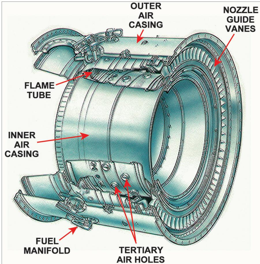
*Figure 16.5* An annular combustion chamber.
