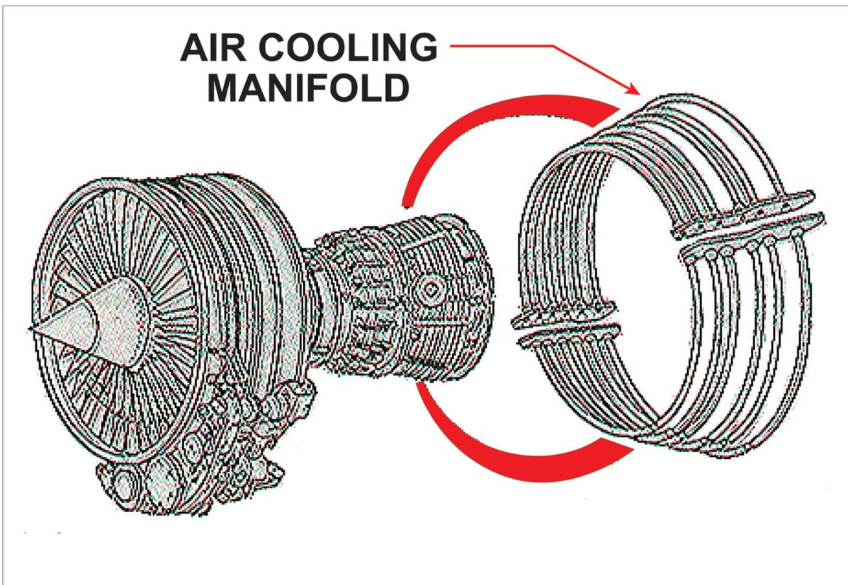
Figure 17.2 Active clearance control used in turbine case cooling.
