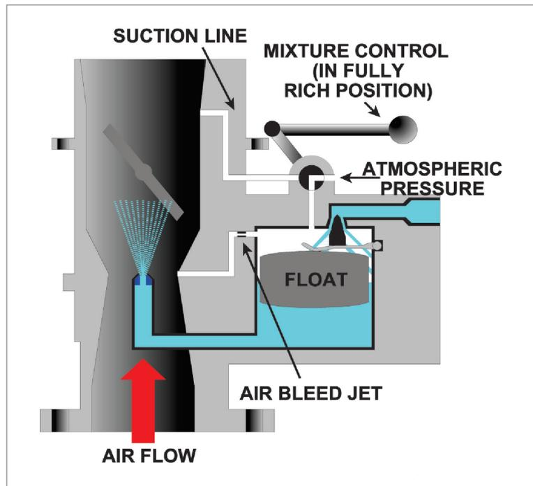
Figure 8.8 An air bleed mixture control.
