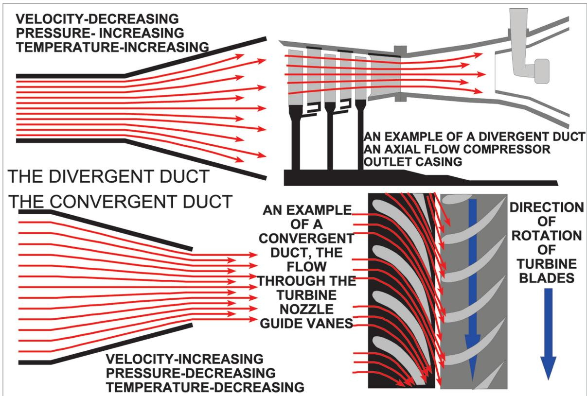
*Figure 13.6 The use of divergent & convergent ducts to control the passage of airflow through the engine.*
