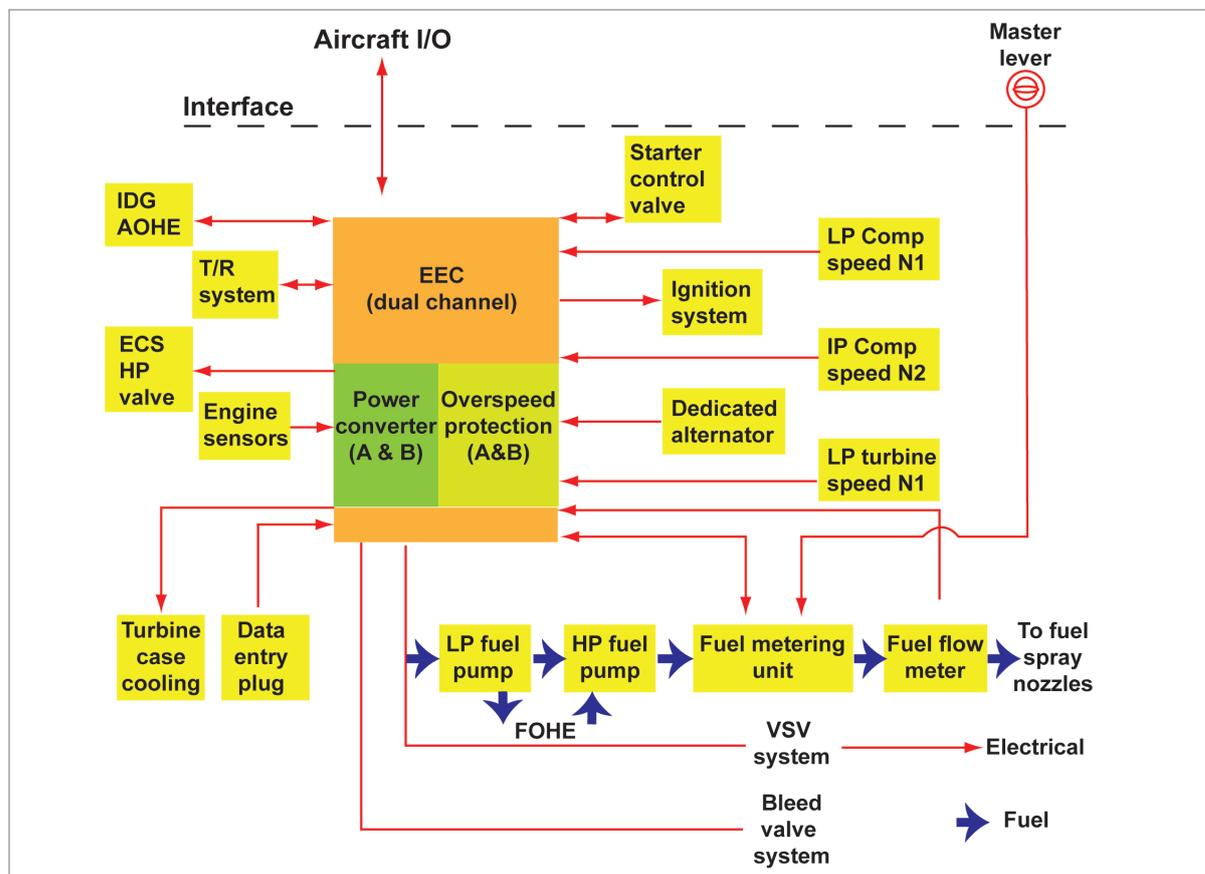
Figure 26.6 A typical FADEC structure
