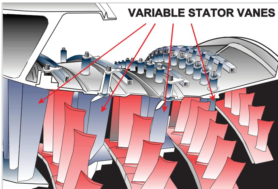
*Figure 15.4 Typical variable stator vanes*
