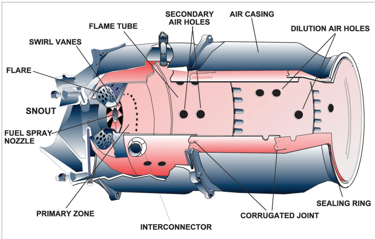
Figure 16.2 An early combustion chamber.
