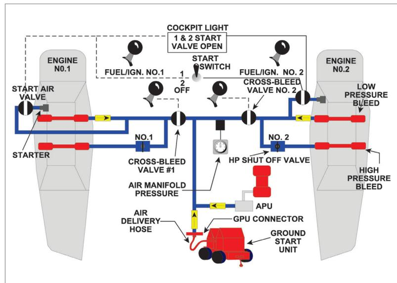
Figure 24.5 Two engine air starter layout
