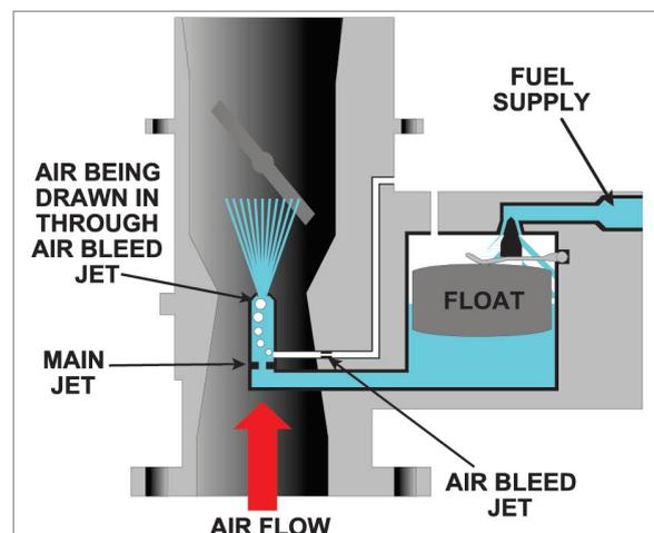
Figure 8.5 The air bleed diffuser.
