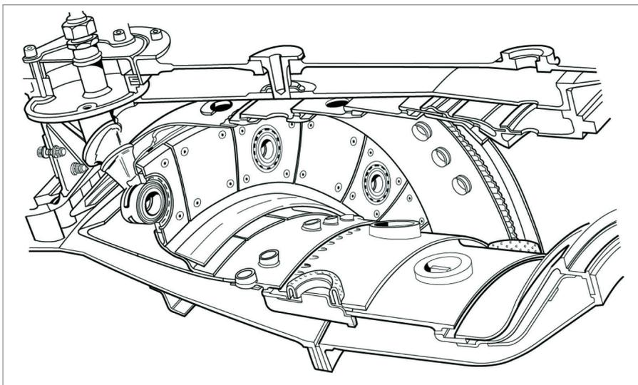
*Figure 16.6* Details of annular combustion chamber (based on an original Rolls-Royce drawing).
