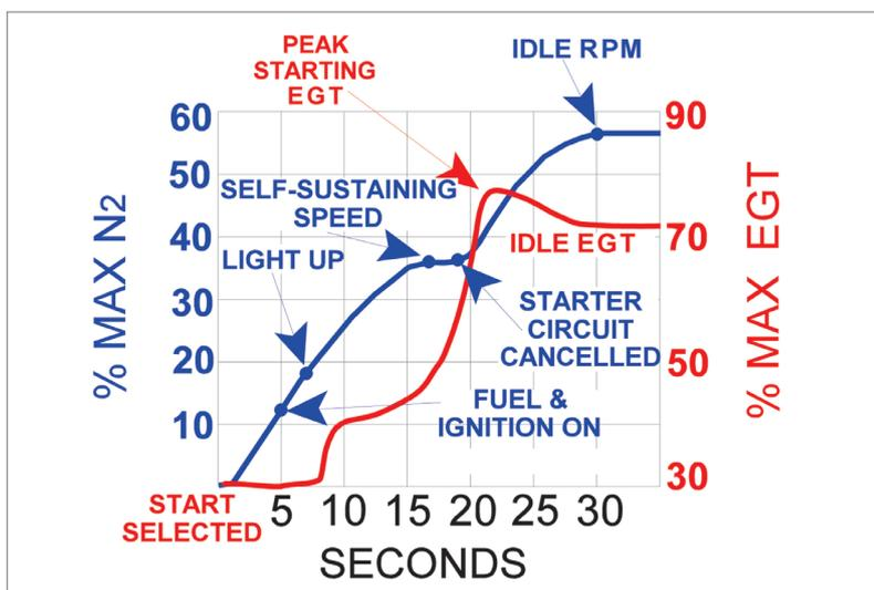
Figure 24.6 RPM/EGT starting relationship
