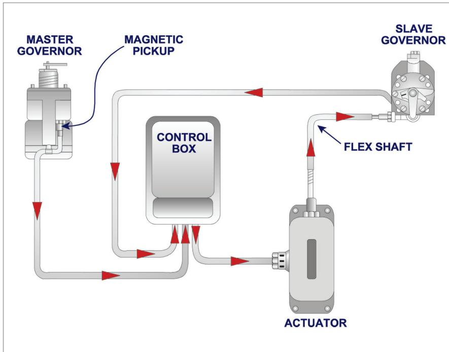
Figure 12.19 Woodward synchronization system for a light twin
