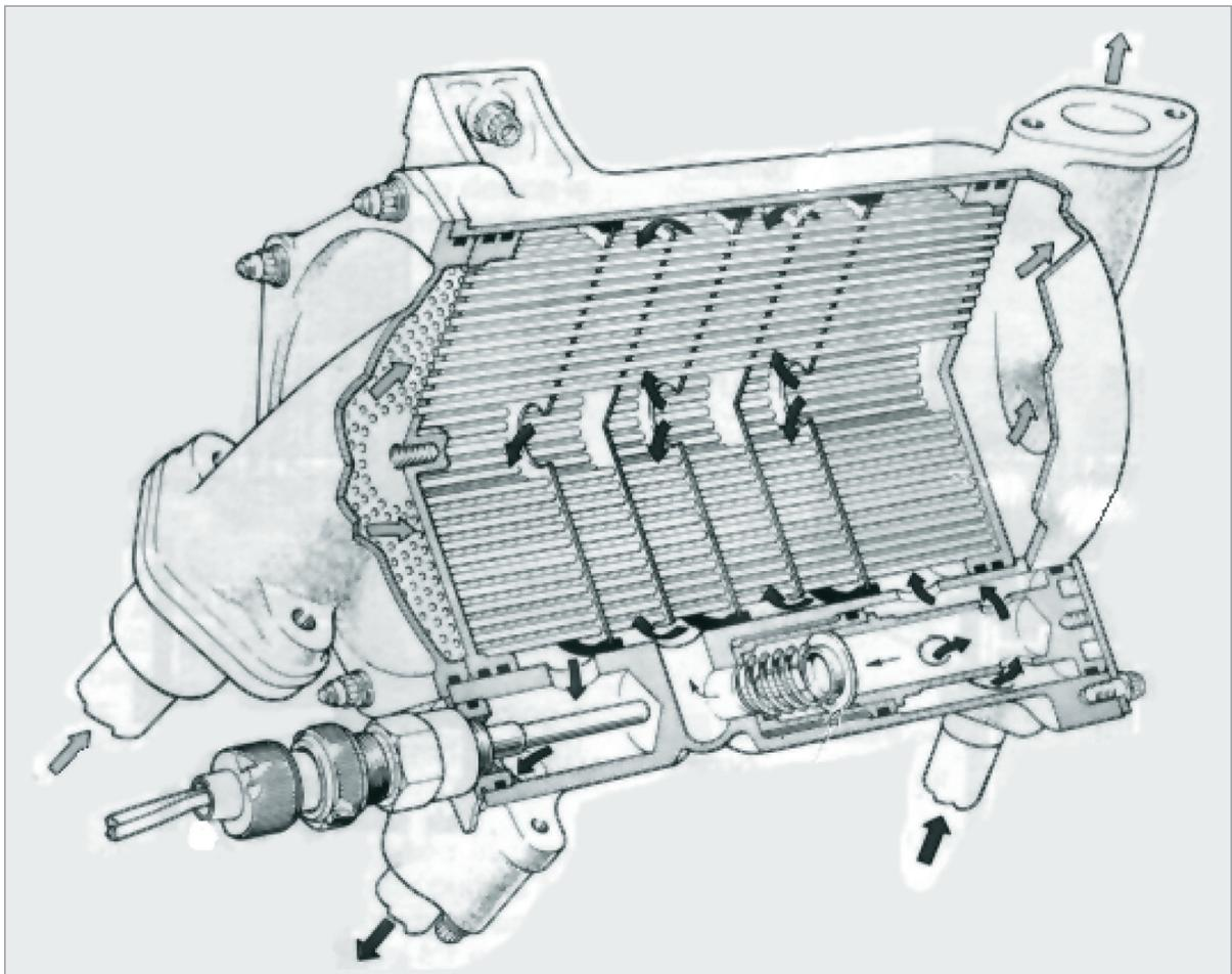
Figure 19.6 A fuel-cooled oil cooler
