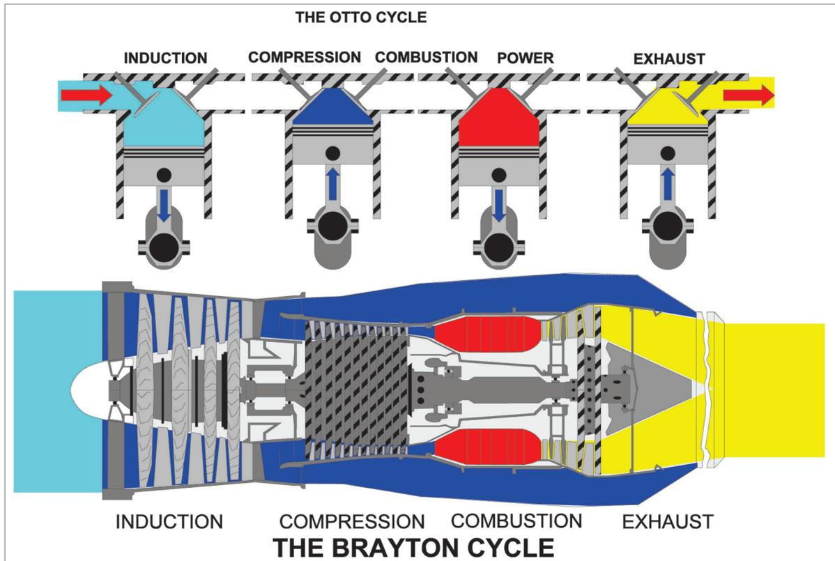
*Figure 13.3 A comparison of the working cycles of the piston engine & the gas turbine engine.*
