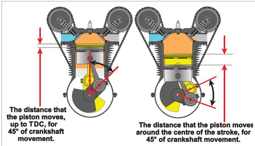
Figure 2.6 Ineffective crank angle
