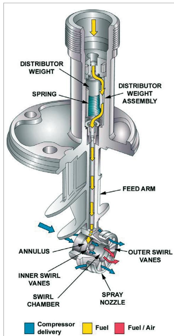
Figure 16.11 An airspray nozzle.
