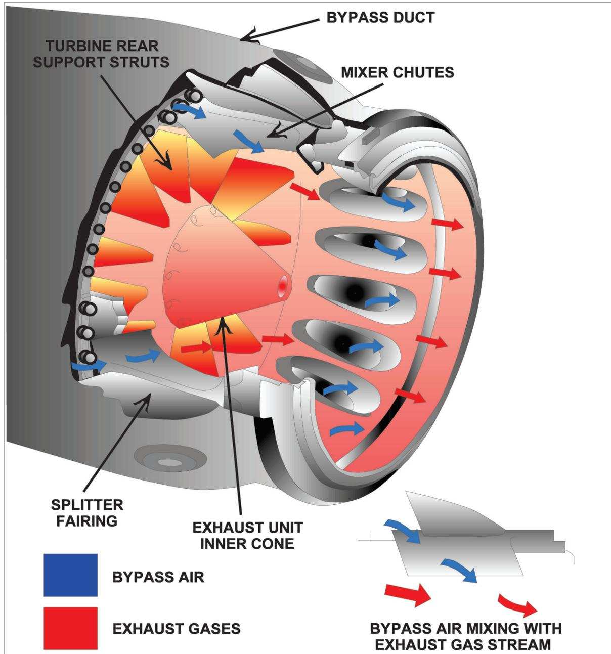
Figure 18.4 A low ratio bypass engine exhaust unit.
