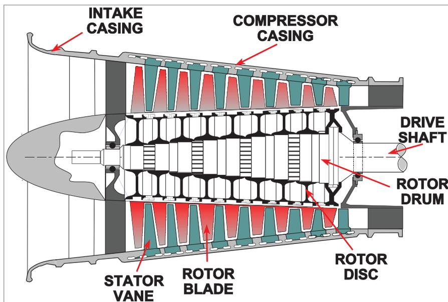
*Figure 15.3 A single spool compressor.*
