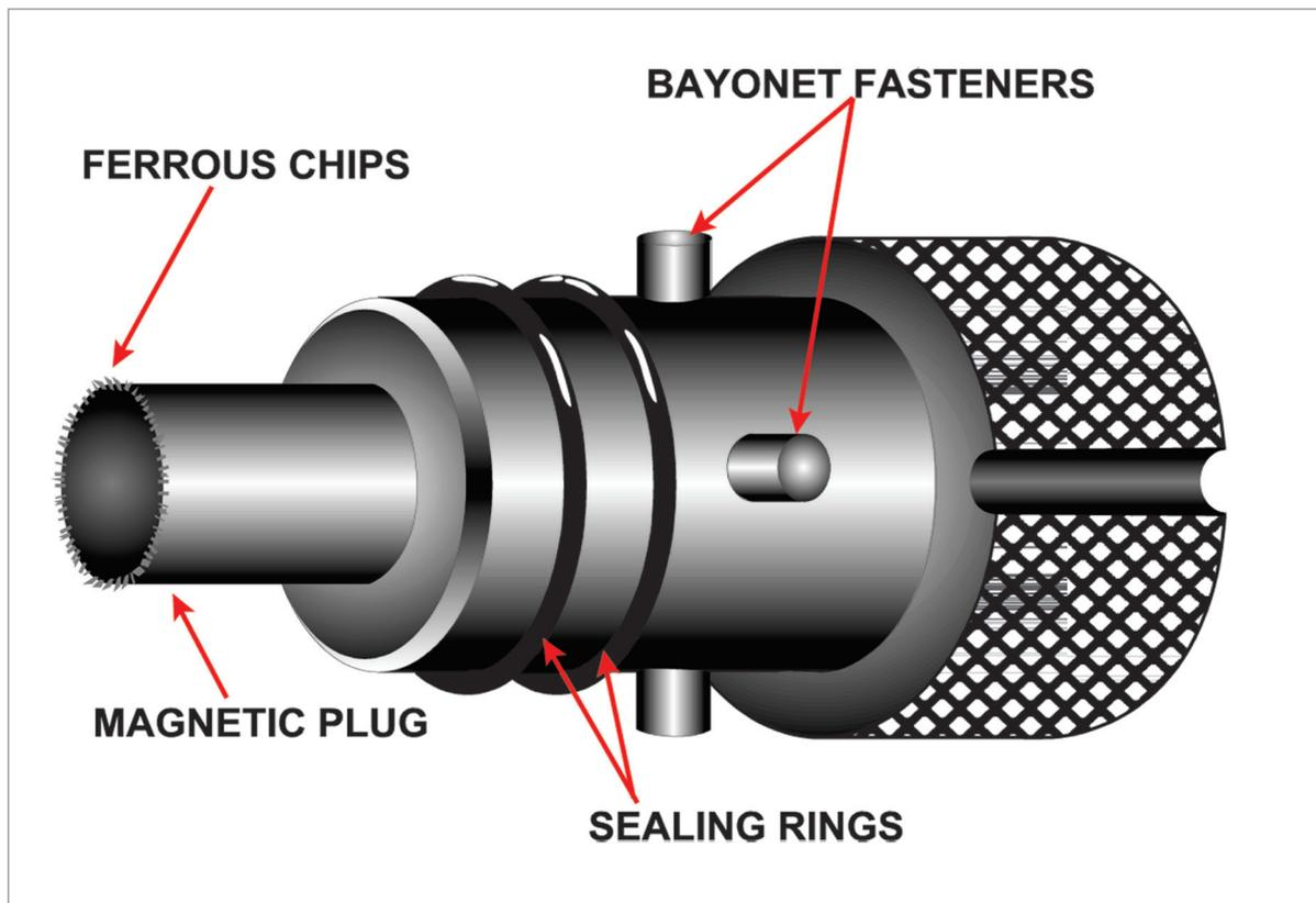
*Figure 19.7 A magnetic chip detector.*
