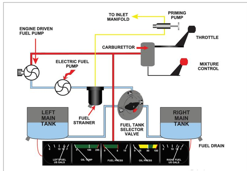
*Figure 8.12 Single-engine light aircraft fuel system & engine priming system.*
