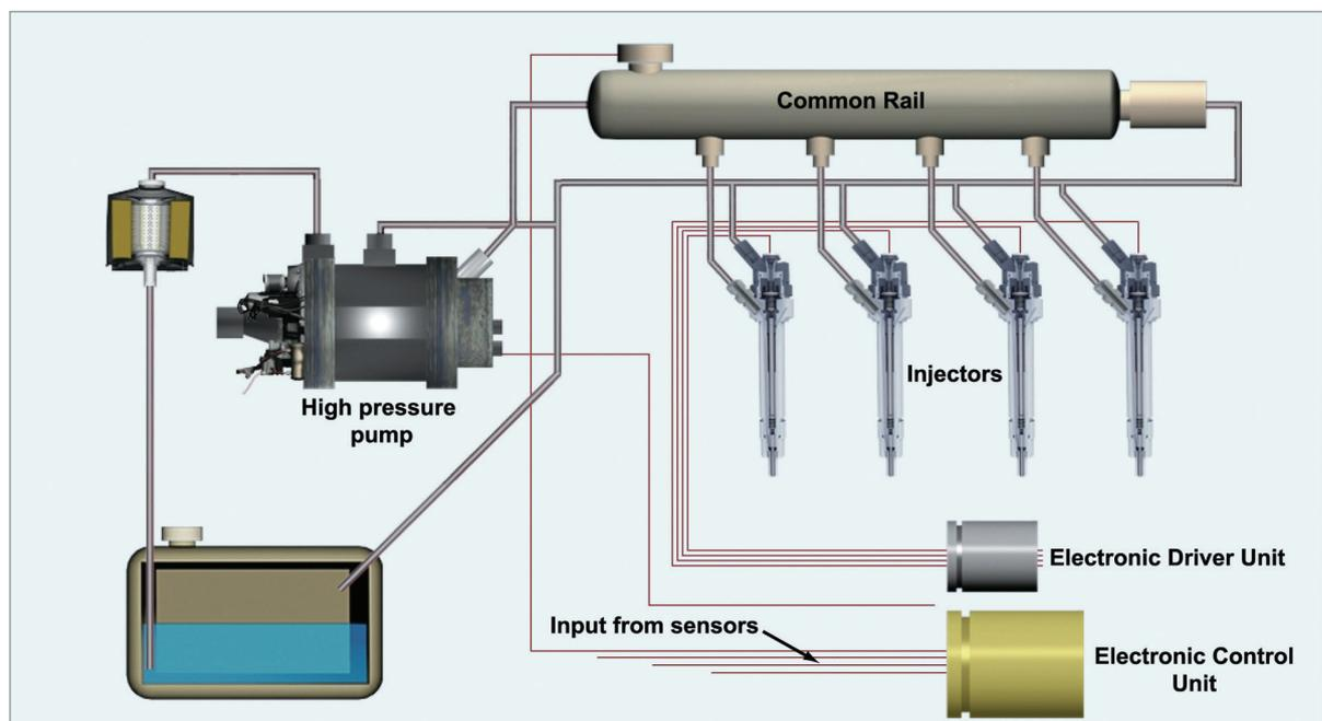
Figure 10.3 A common rail system.
