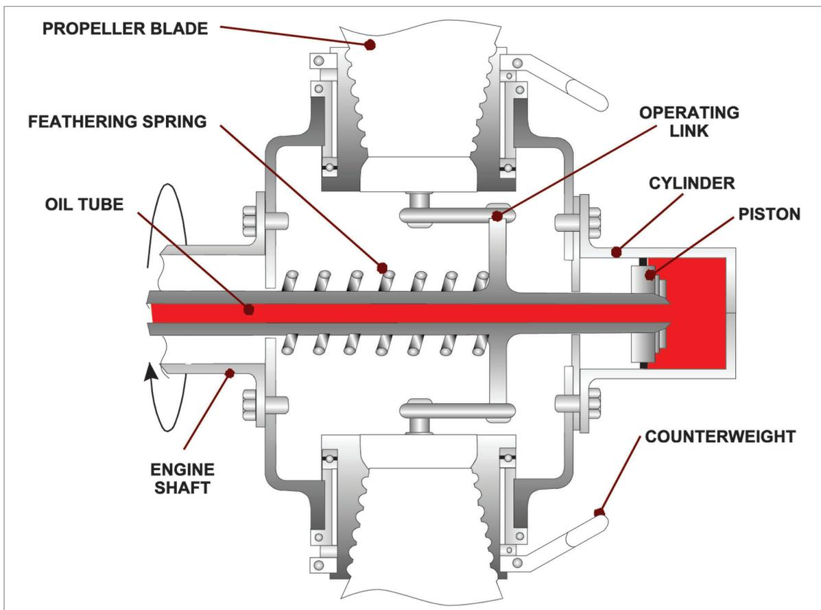
Figure 12.9 The single acting propeller
