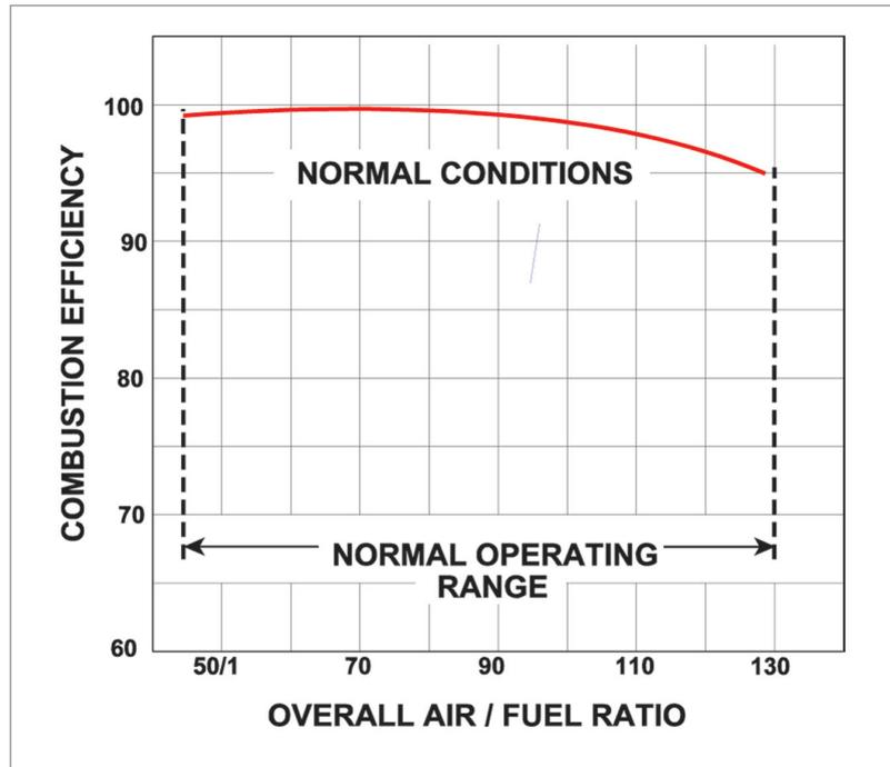
Figure 16.9 Combustion Efficiency and Air/Fuel Ratio.
