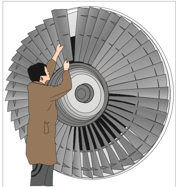
Figure 15.9 A high bypass ratio engine low pressure compressor or fan.
