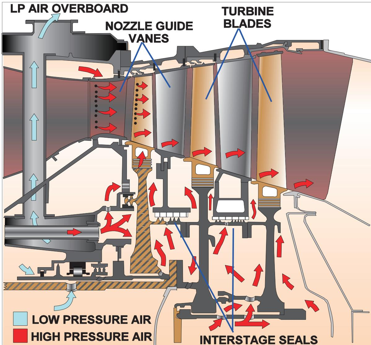
Figure 27.3 Cooling & sealing within the turbine area.
