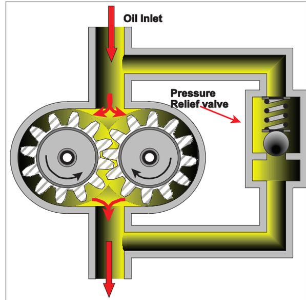
Figure 3.2 Spur gear pump
