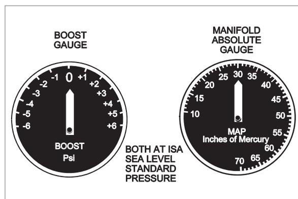
Figure 11.2 Manifold pressure indications.
