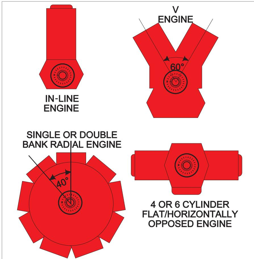
Figure 2.1 Engine Layouts
