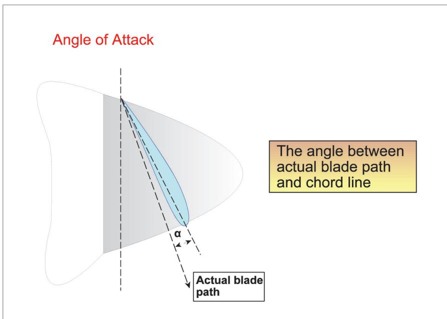
Figure 12.4 Angle of attack
