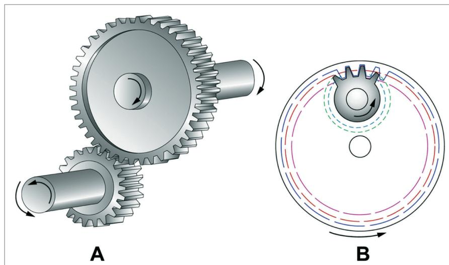
Figure 12.22 Two types of spur type reduction gear arrangement
