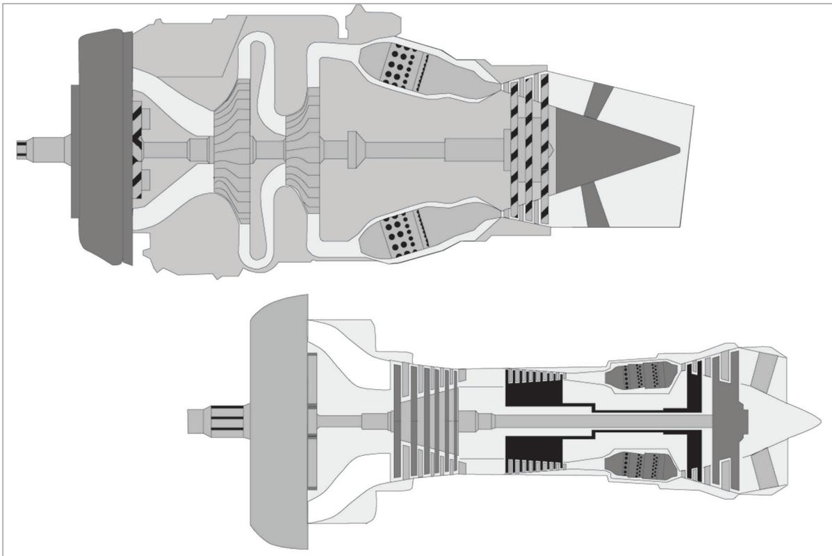
Figure 13.8 Centrifugal and axial compressor turboprop engines.
