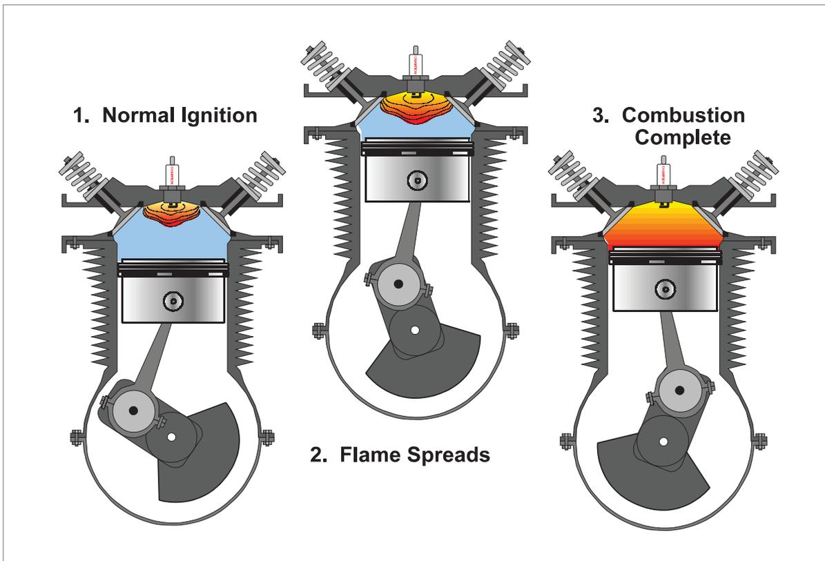
Figure 6.1 Normal combustion.
