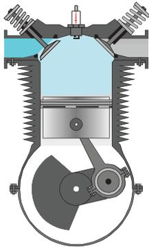
**1. The inlet valve is open, permitting flow from atmosphere, through the carburettor into the cylinder.**
