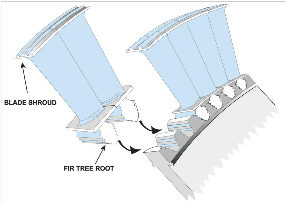
Figure 17.7 Fir tree root turbine blade attachment.
