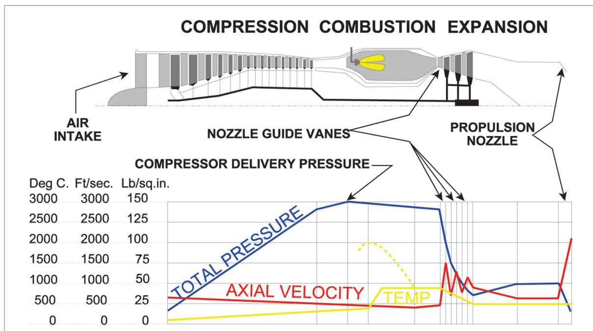
Figure 13.5 Changes in pressure, temperature & velocity in a single spool axial flow engine.
