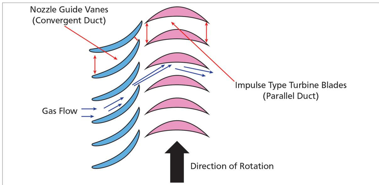
Figure 17.5 and Figure 17.6 How the twist of the blade changes it from impulse to reaction.
