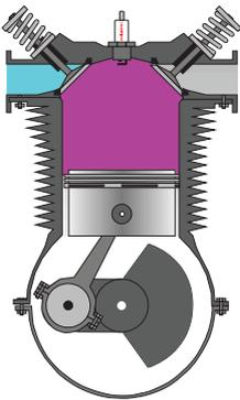
**2. Both of the valves are closed trapping the induced mixture in the cylinder. The piston is moving up. The cylinder volume is decreasing. The cylinder pressure is increasing. The temperature of the charge is increasing. The mass of the charge is now fixed.**
