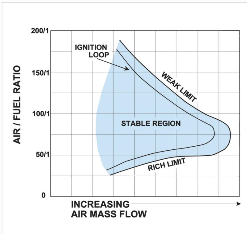
Figure 16.7 A typical combustion stability loop.
