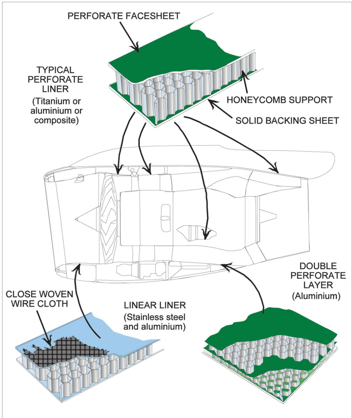
Figure 18.8 The types of materials used for noise suppression & their locations.
