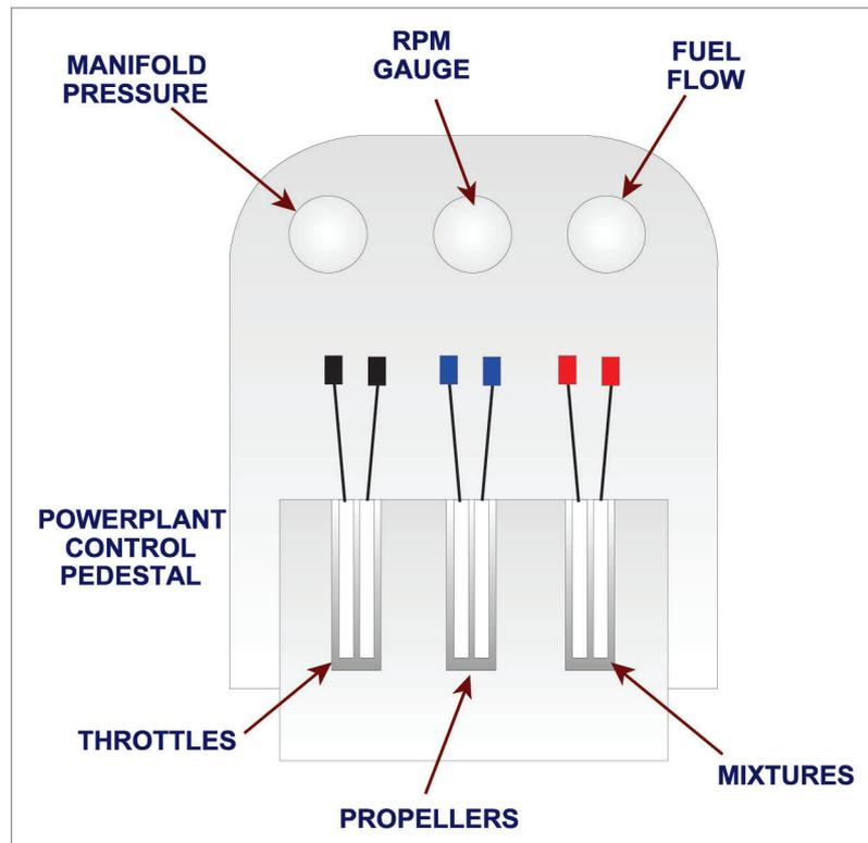
Figure 12.25 A typical light twin powerplant controls arrangement
