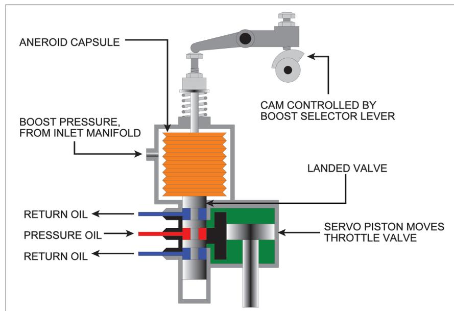
*Figure 11.11* An automatic boost control unit.
