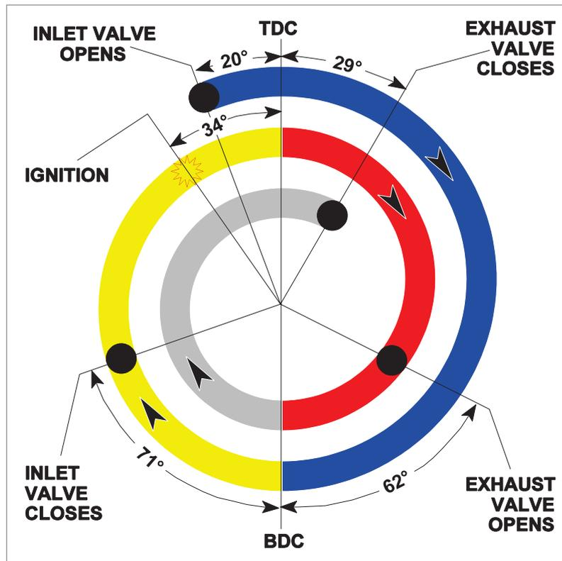
Figure 2.5 A practical valve and ignition timing diagram
