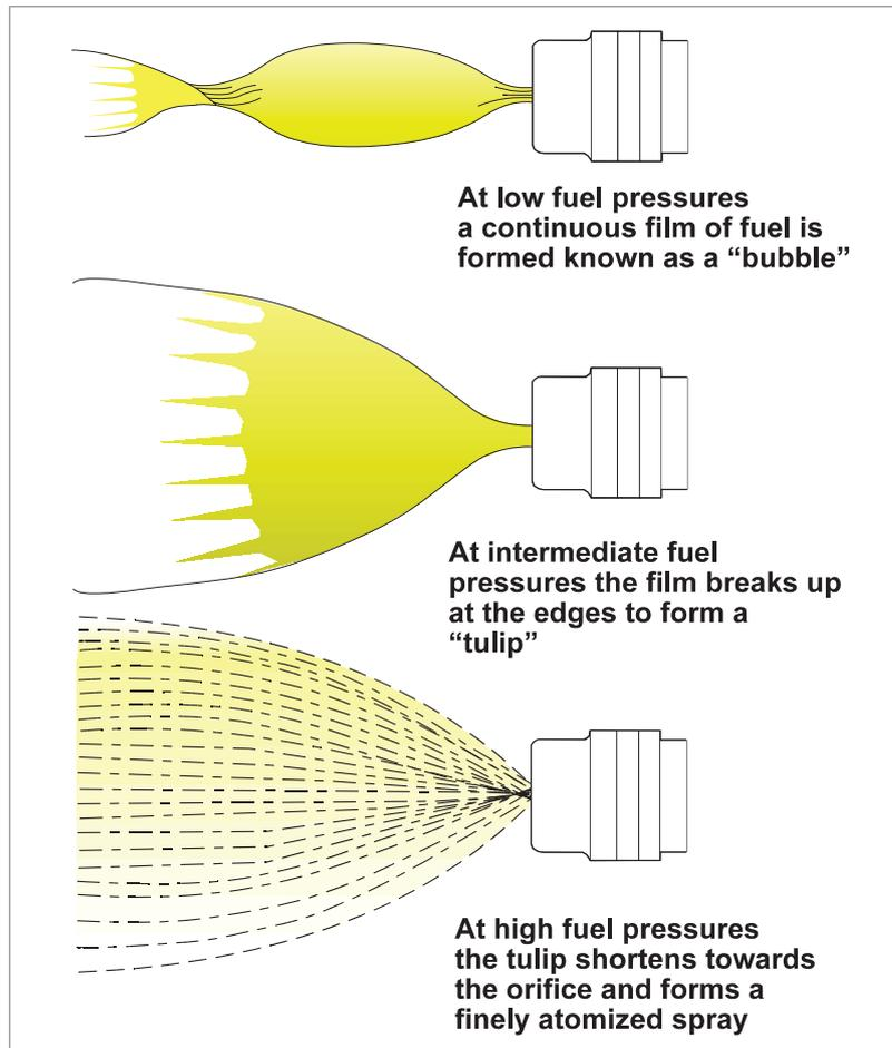
Figure 16.10 Fuel spray patterns at various pressures.
