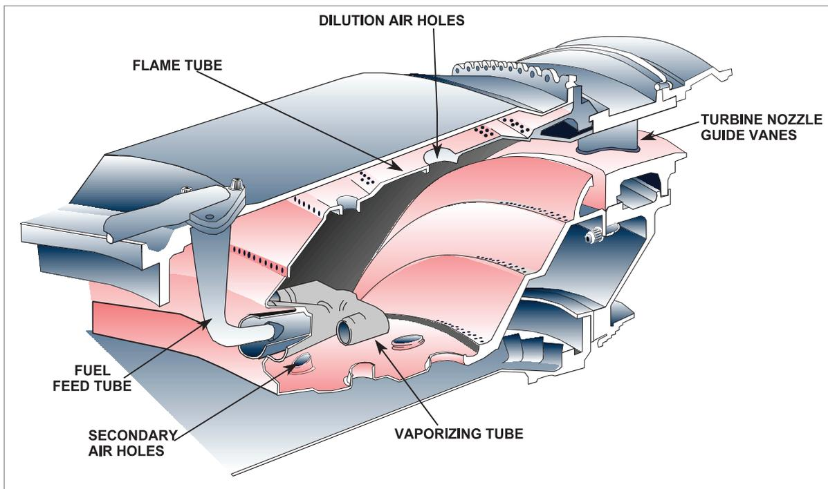
*Figure 16.13* The vaporizing method of fuel feed.
