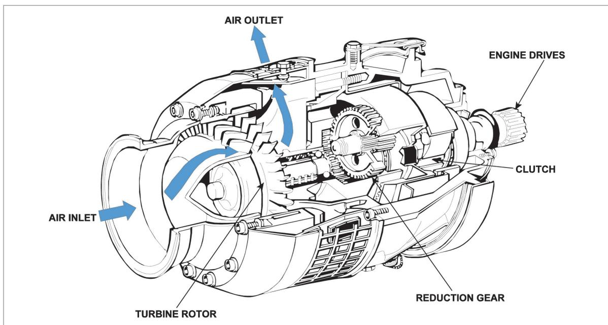
Figure 24.4 An air starter motor
