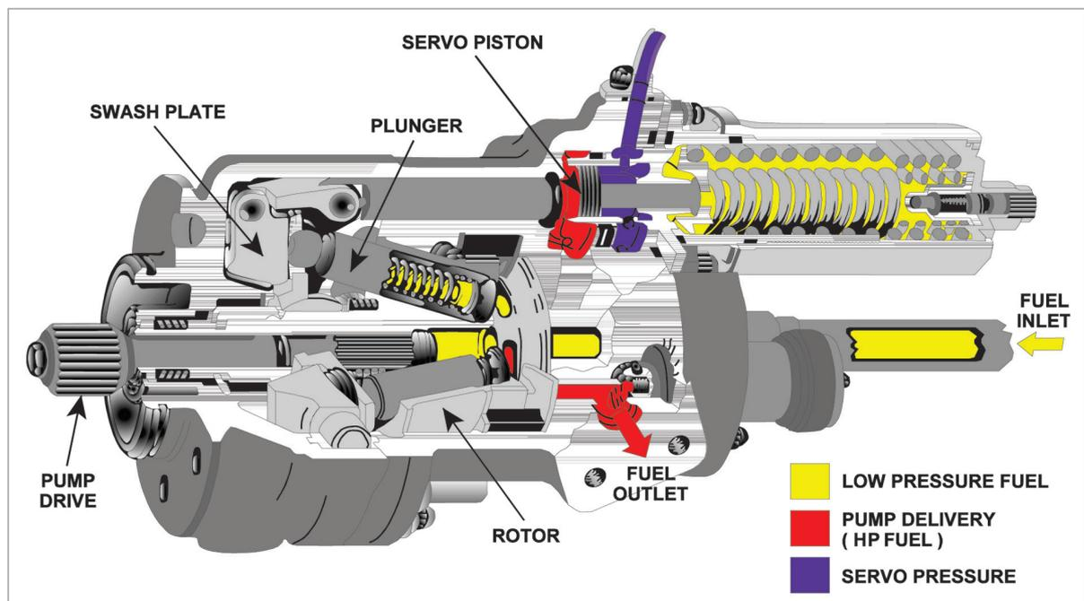
Figure 26.2 Axial piston type fuel pump (based on an original Rolls Royce drawing)
