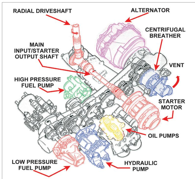
Figure 22.4 An external gearbox showing various accessories.
