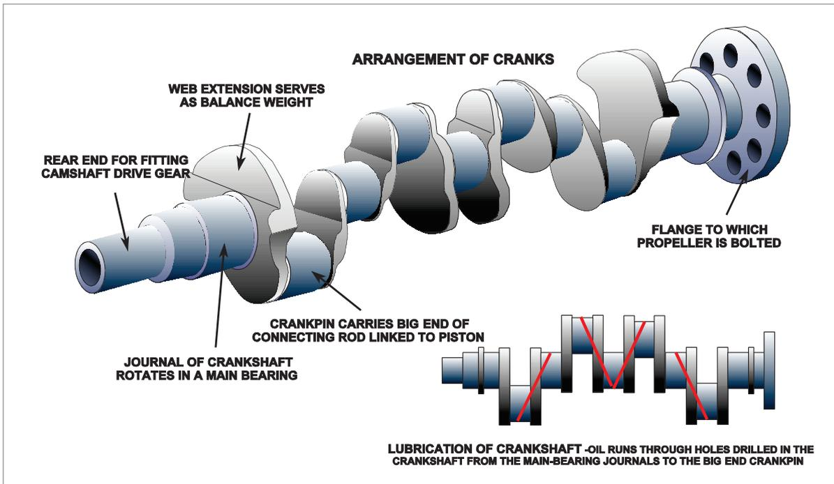
Figure 2.12 A four cylinder crankshaft
