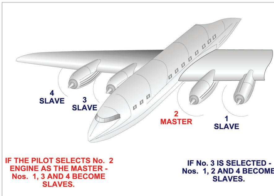
Figure 12.20 The master engine arrangement of a transport aircraft
