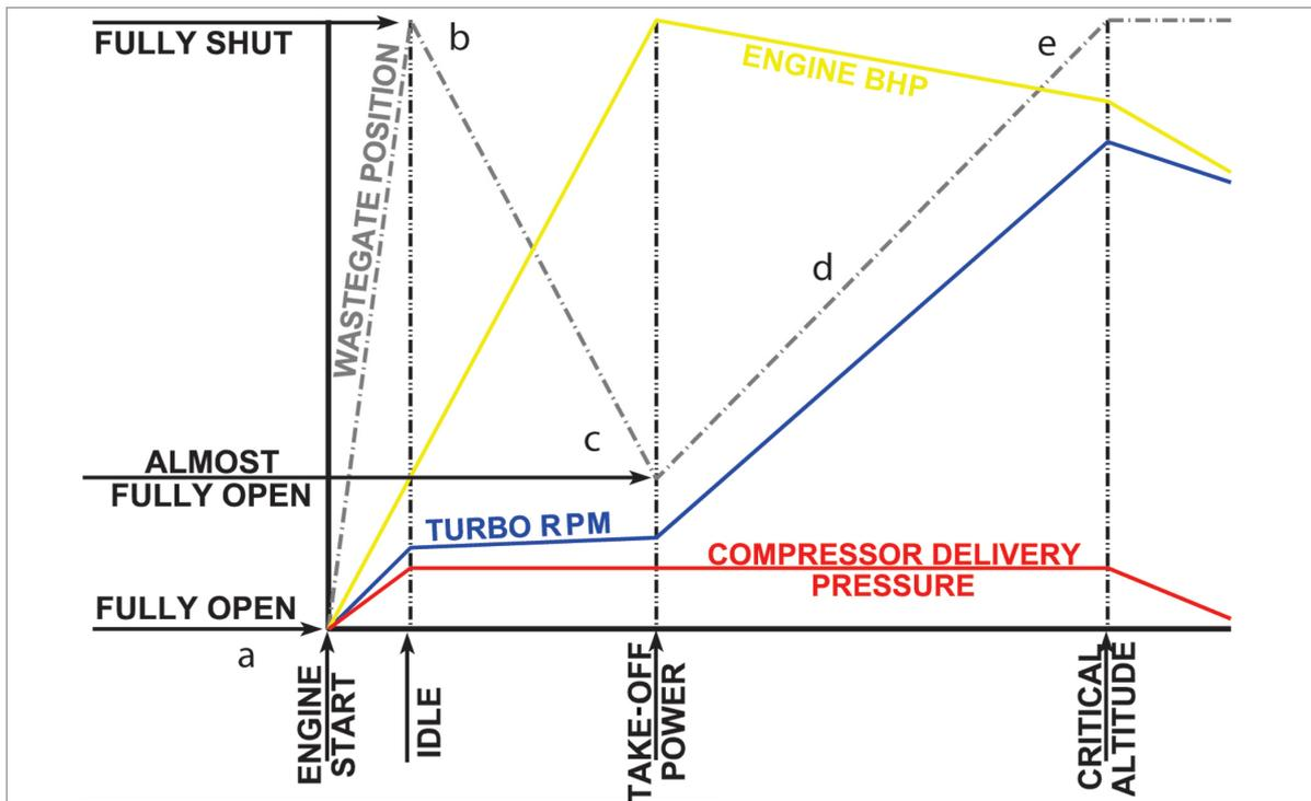
Figure 11.5 The relationship of wastegate position, engine power, manifold pressure & turbocharger rpm to each other.
