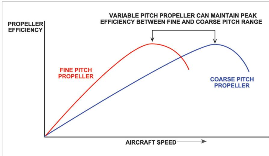
Figure 12.7 Propeller efficiency curves
