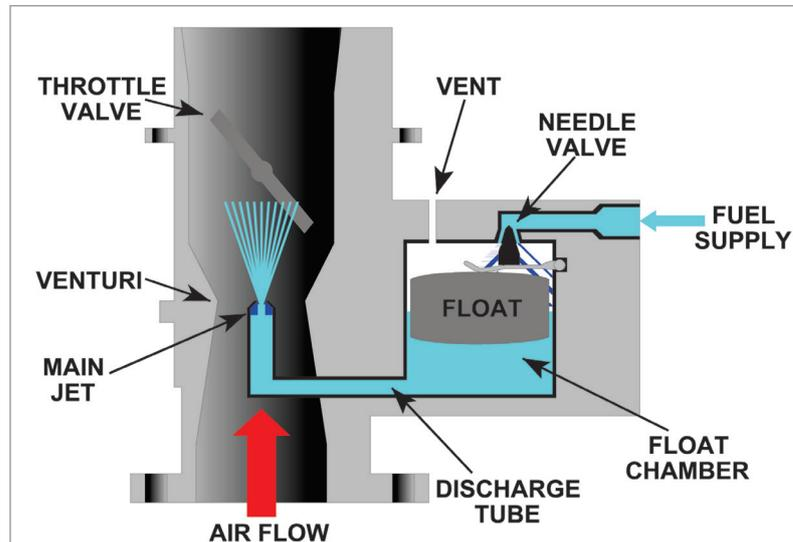
Figure 8.2 A simple float chamber carburettor.
