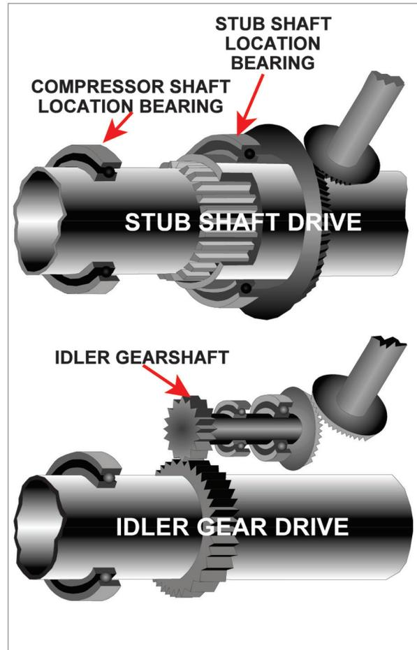
*Figure 22.2 Two methods of gear drive from the compressor shaft.*
