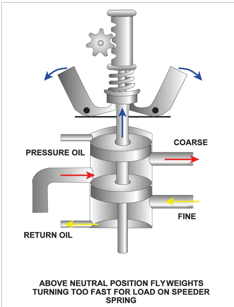
Figure 12.13 Overspeed condition.
