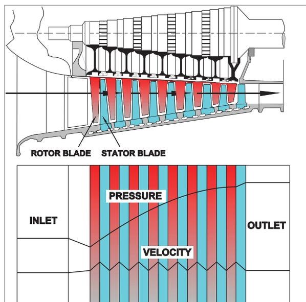
Figure 15.2 The changes in pressure & velocity through an axial flow compressor.
