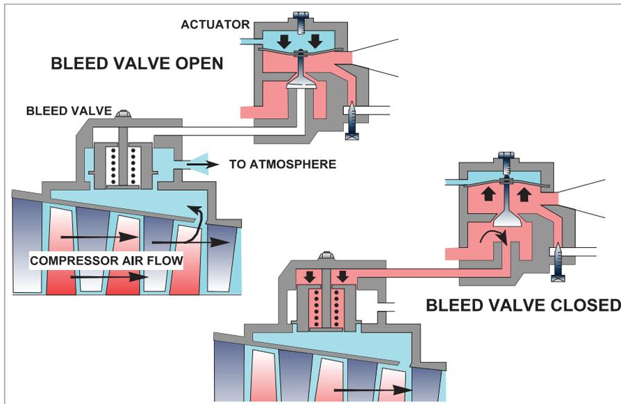
Figure 15.5 The operation of a compressor bleed valve.
