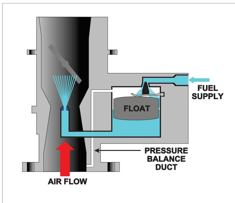
*Figure 8.3 The pressure balance duct.*
