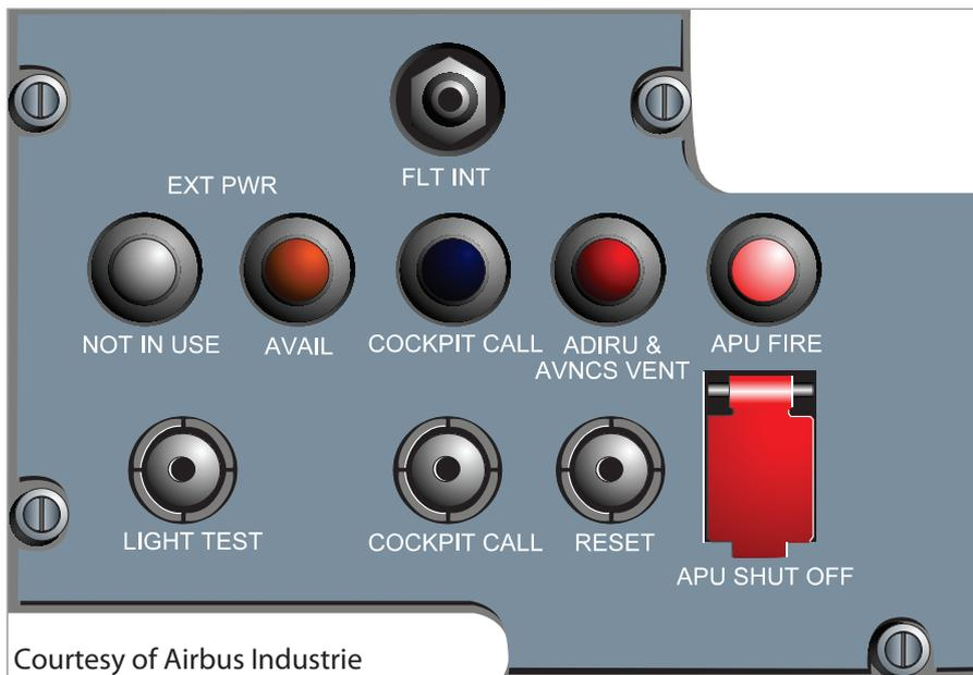
Figure 24.3 External APU control panel
