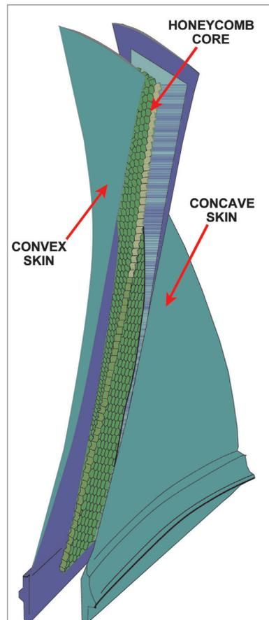
*Figure 15.10 Wide chord fan blade construction.*
