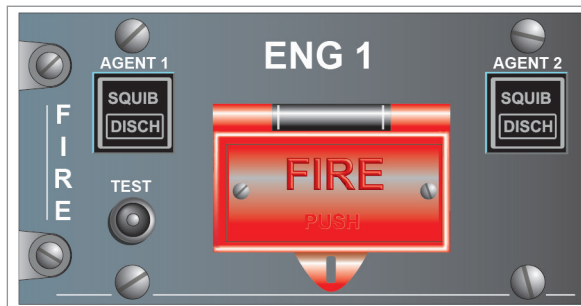
Figure 15.7 Cockpit overhead engine fire panel
