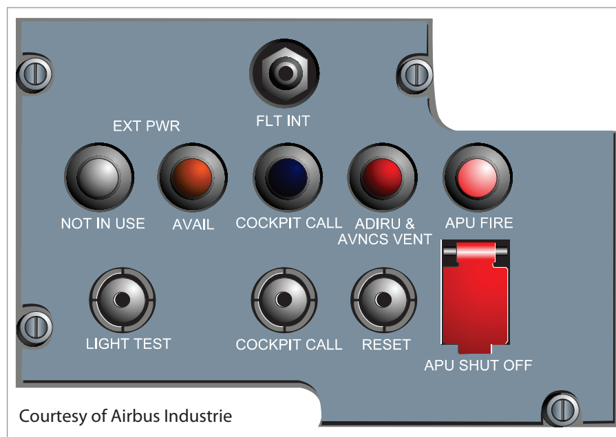
Figure 15.11 External APU fire control panel (Airbus)
