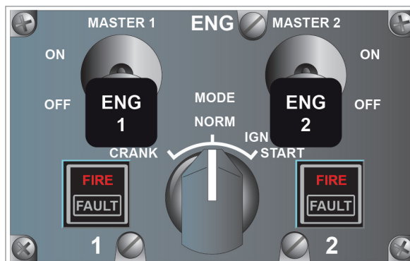
Figure 15.8 Pedestal engine and fire control panel
