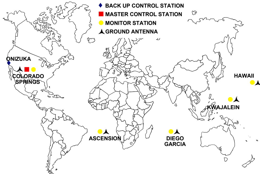
Figure 19.8 GPS Operational Control Segment
