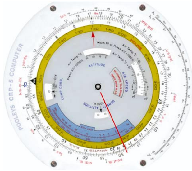
Figure 6.12 TAS corrected for compressibility
