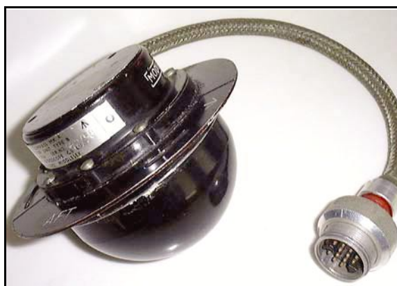
Figure 32.3 A Magnetic Detector Unit
