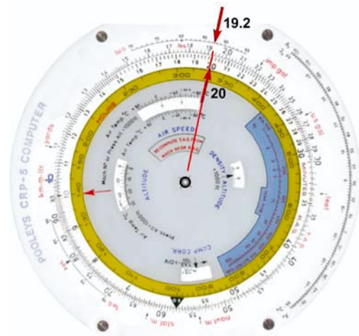
Figure 6.18 True Alt (outer scale) against Indicated Alt (inner scale)
