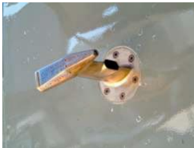
Figure 3.6 A TAT Probe Fitted to a Boeing 737
