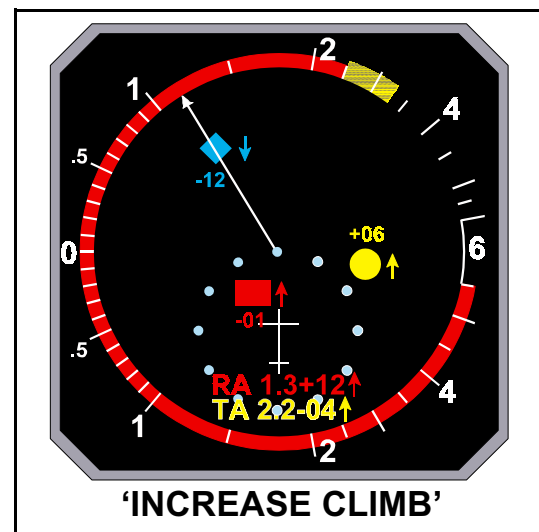
Figure 36.14 No Bearing RA and TA
