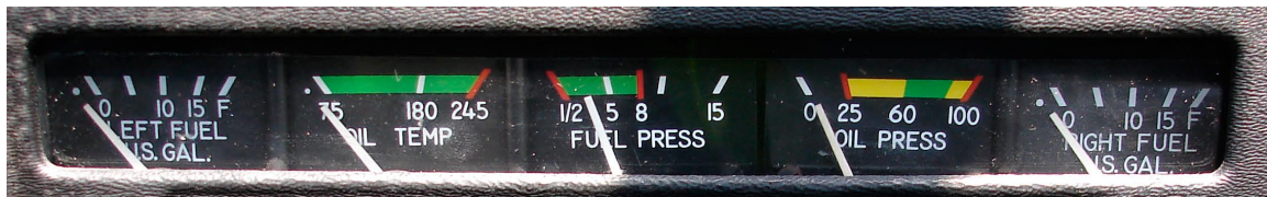
Figure 1.13 Red, yellow and green operating ranges.
