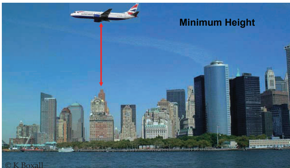
Figure 6.3: An aircraft must be flown at a height from which, in the event of an emergency, a landing can be made without undue hazard to persons or property on the surface.
